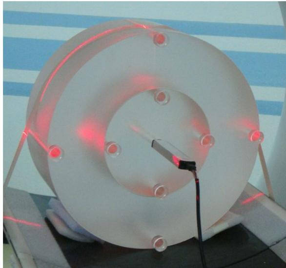
**Figure 3.6 PMMA phantoms with chamber insert at center**
