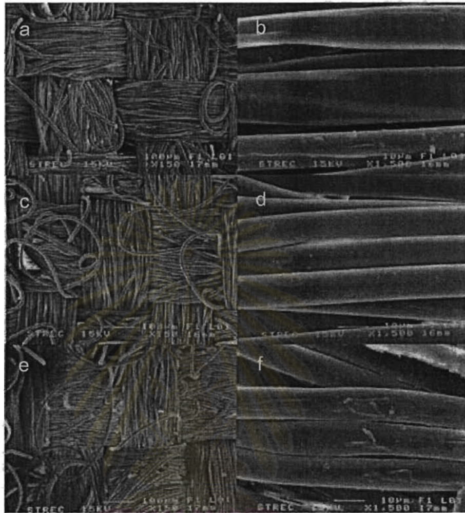
Figure 4.34 SEM photographs at x150 (left) and x1,500 (right) of untreated control (a and b), buffer (c and d) and 0.5 U/ml enzyme (48 h) (e and f).
