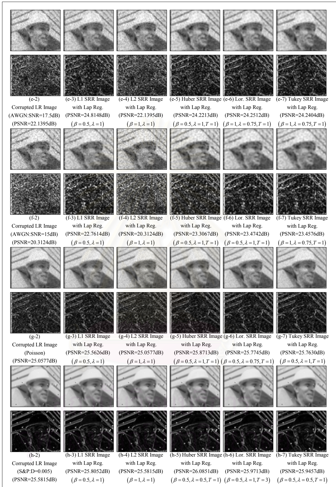
Figure 4.18 : The experimental result of the SRR algorithm using proposed robust estimation technique with classical registration (Foreman Sequence : The 110 th frame)) (Con.)
