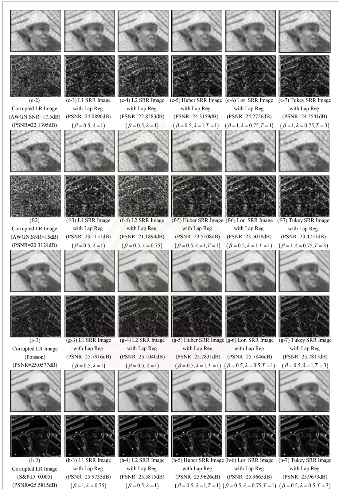
Figure 4.22 : The experimental result of the SRR algorithm using proposed robust estimation technique with proposed registration (Foreman Sequence : The 110 th frame) (Con.)
