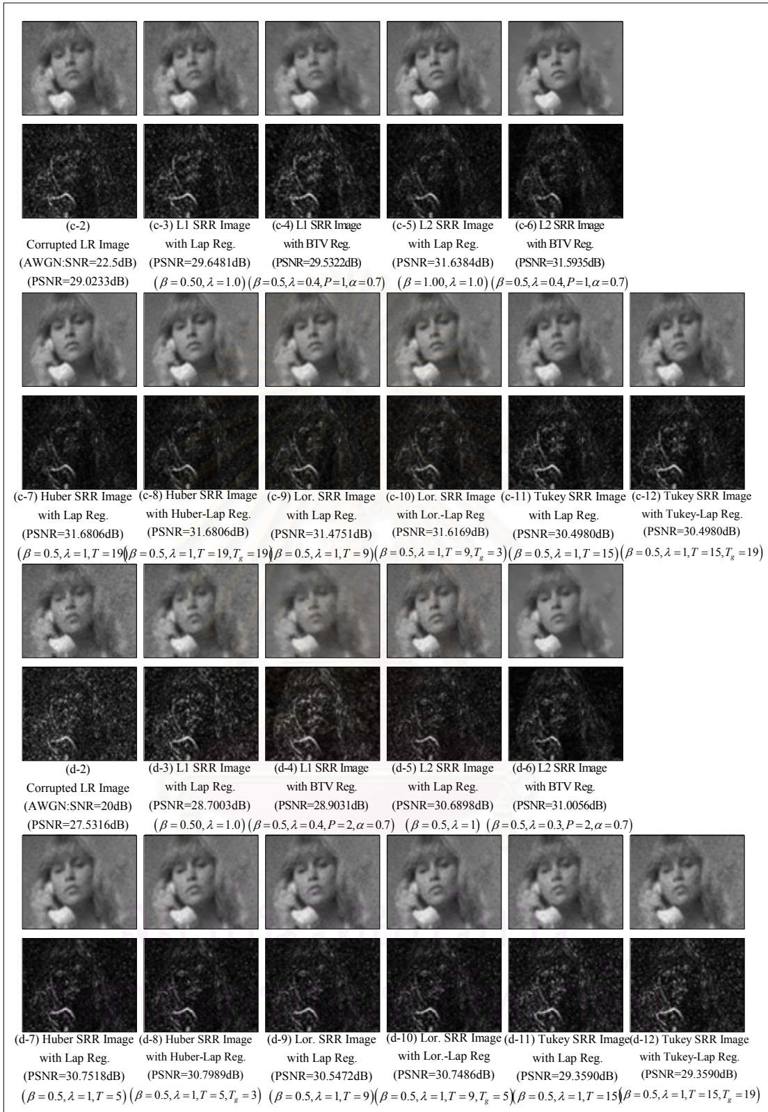
Figure 4.13 : The experimental result of SRR algorithm using the proposed robust estimation technique (Susie Sequence : The 40th Frame) (Con.)
