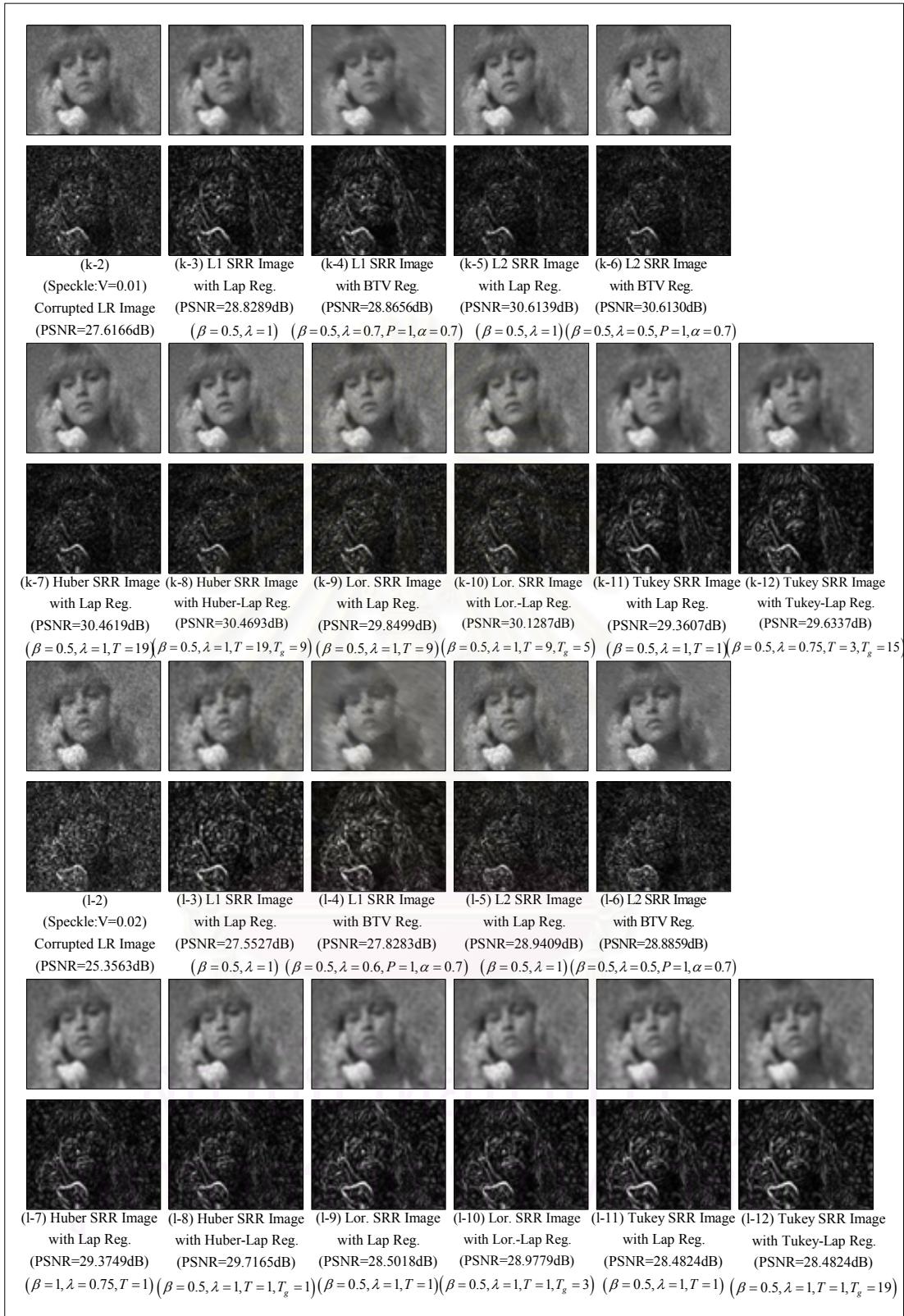
Figure 4.13 : The experimental result of SRR algorithm using the proposed robust estimation technique (Susie Sequence : The 40th Frame) (Con.)
