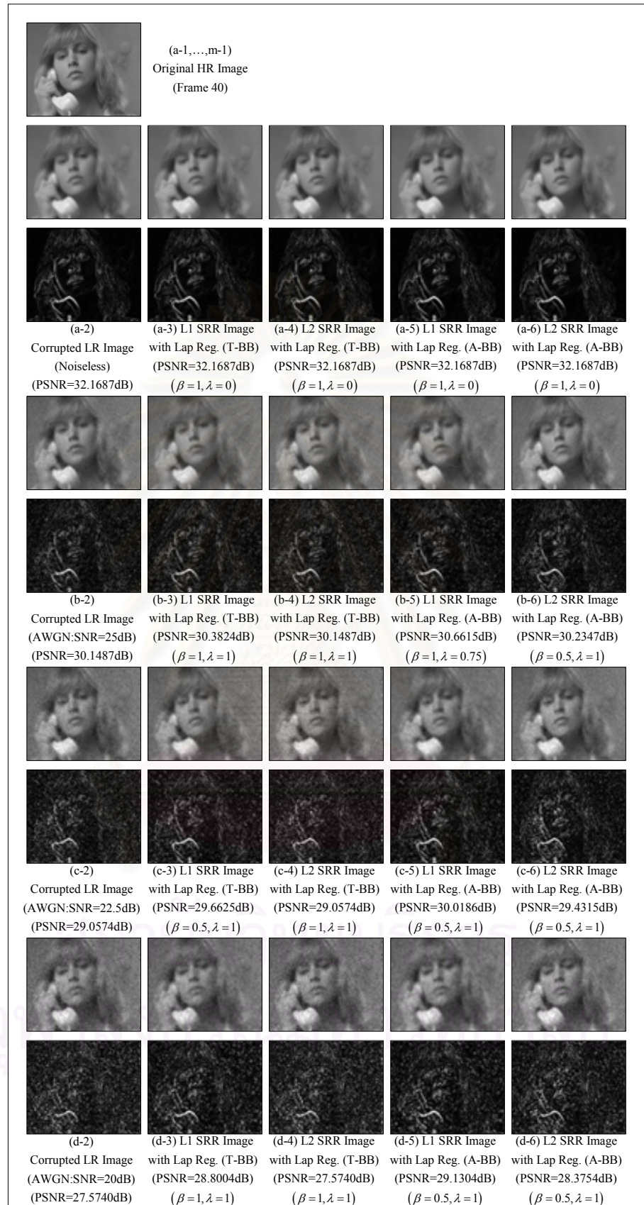
Figure 4.8 : The experimental result of SRR algorithm using the proposed Registration (Susie Sequence : The 40 th Frame)
