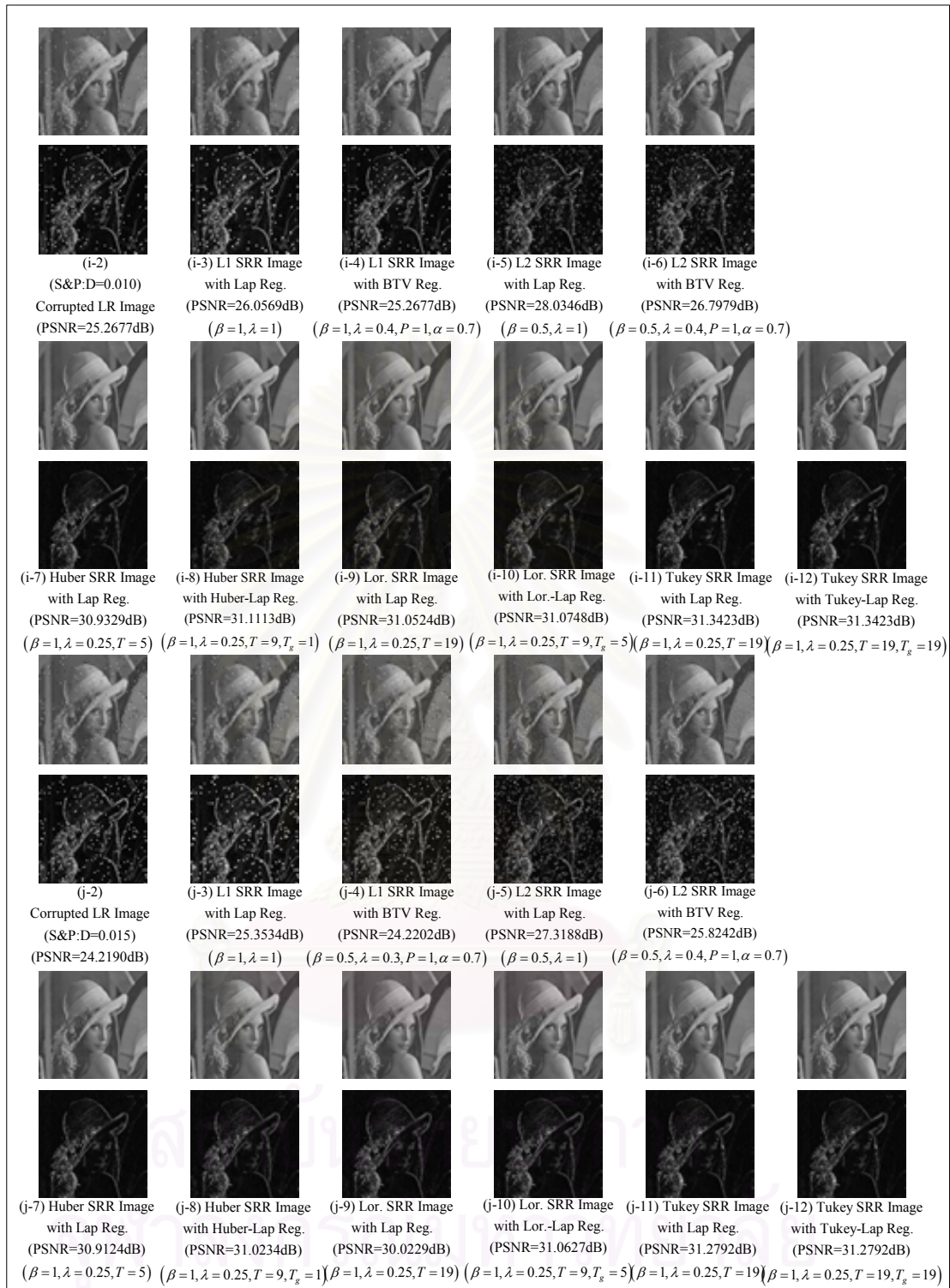
Figure 4.14 : The experimental result of SRR algorithm using the proposed robust estimation technique (Lena : The Standard Image) (Con.)
