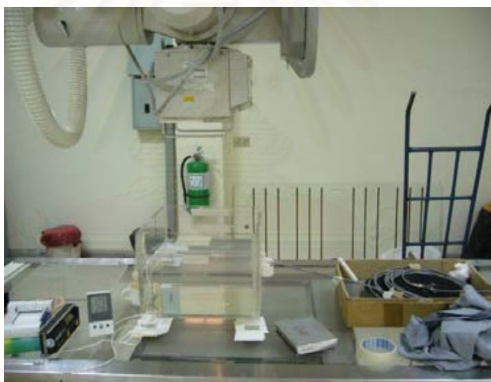
Figure 3.13 The setup of thermoluminescent dosimeter for linearity dose response
