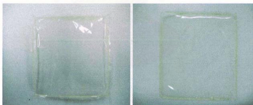
Figure 4.1 Unmodified chitosan film cast with acetic acid (left) and lactic acid (right).
