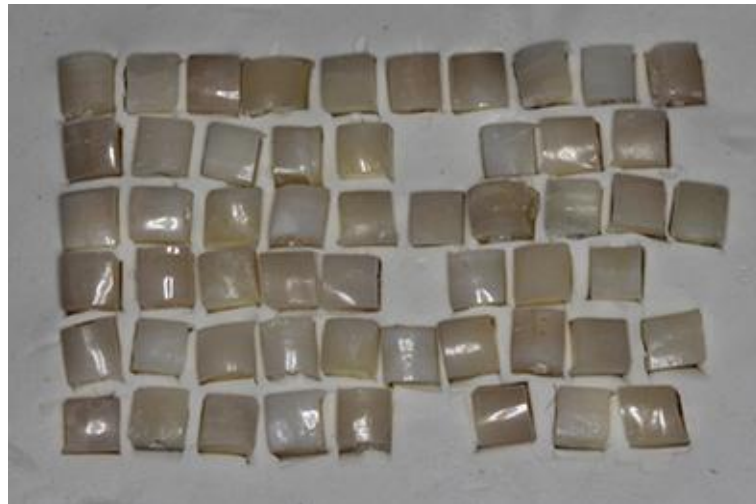
Figure 3 Mounted specimens in plasticine
