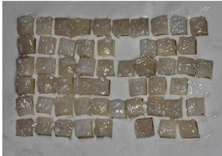
Figure 4 Applied bleaching gel on each specimen
