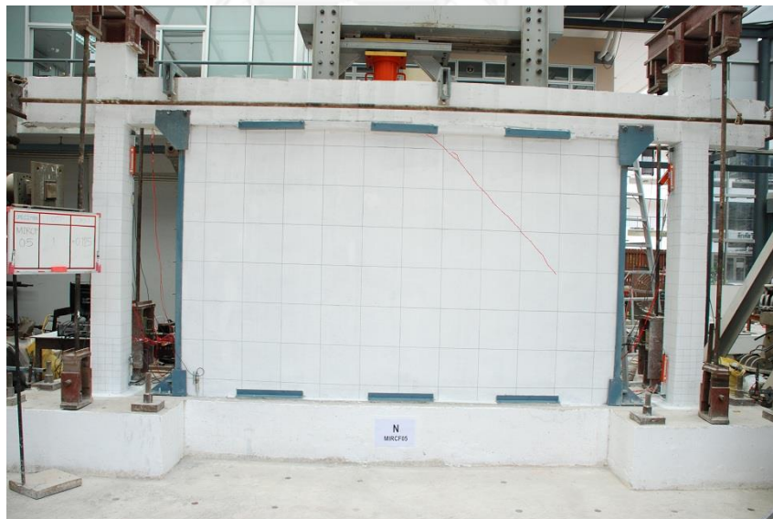
Figure 4-18. Damage condition of specimen MIRCF04 at 0.125% drift
