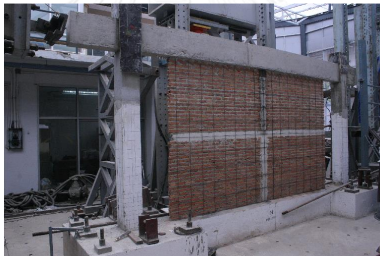
CHULALONGKORN UNIVERSITY Figure 3-14. URM of test specimen MIRCF04 reinforced with steel wire mesh
