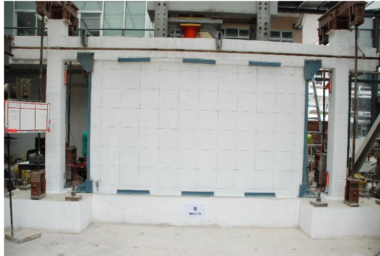
Figure 3-15. Test specimen MIRCFO4 with small angles to prevent out-of-plane deformation
