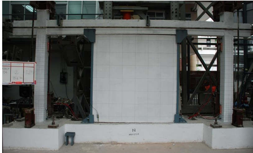
Figure 4-49. Retrofitted specimen MIRCFO3 at LS Performance Level
