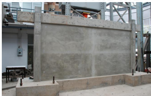
Figure 3-9. Construction sequence of the test specimen MIRCFO1: (a) RC frame casting; (b) URM panel assembly; and (c) URM panel plastering
