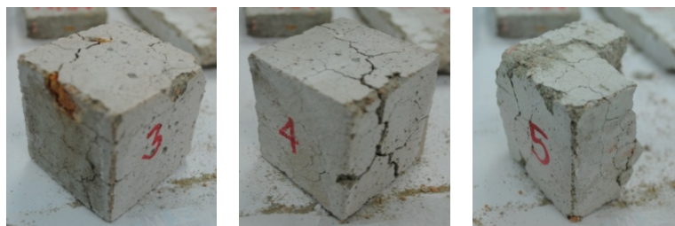
Fig. 4 – 8 Deterioration of air – dried condition standard cube specimens
