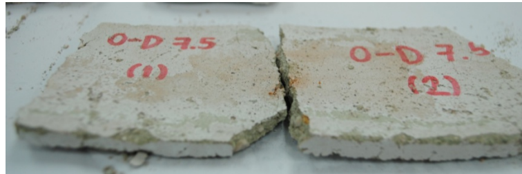
Fig. 4 – 11 Deterioration of oven – dried condition specimen 7.5 mm thick
