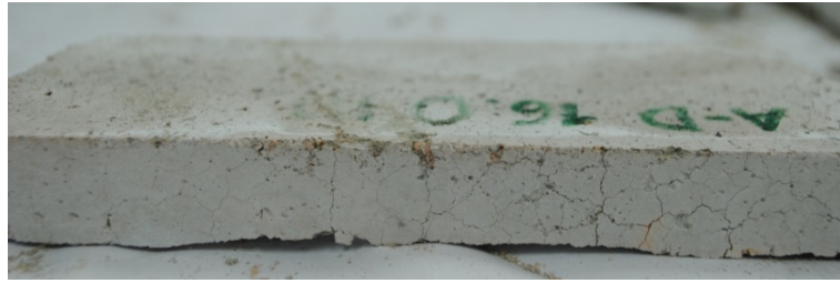
Fig. 4 – 5 Deterioration of air – dried condition specimen 16.0 mm thick
