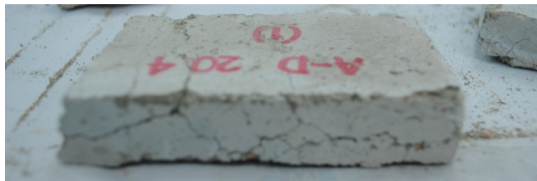
Fig. 4 – 7 Deterioration of air – dried condition specimen 20.4 mm thick
