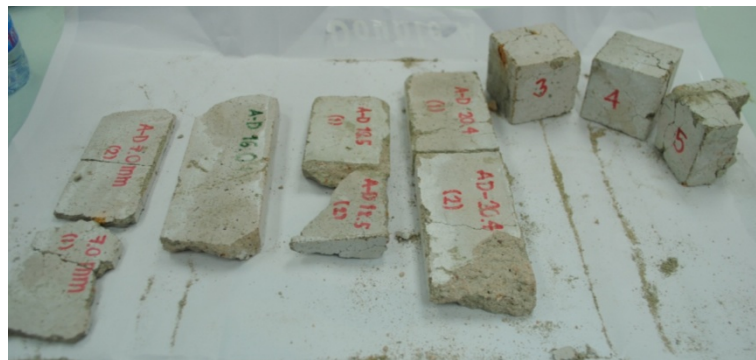
Fig. 4 – 3 Air – dried condition specimens after test
