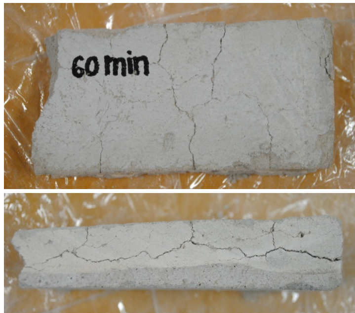
Fig. 4 – 17 Cracked samples after 60 minutes of exposure
