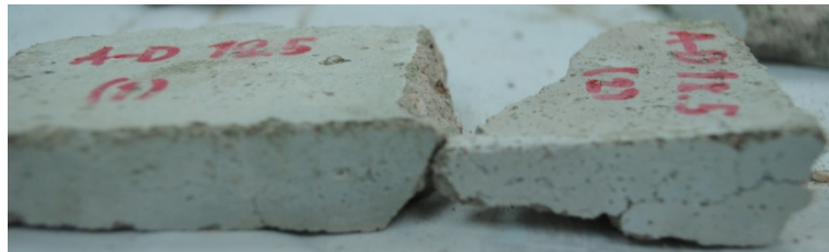
Fig. 4 – 6 Deterioration of air – dried condition specimen 18.5 mm thick
