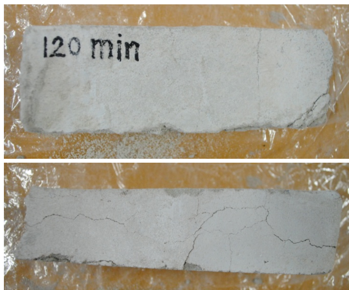
Fig. 4 – 18 Cracked samples after 120 minutes of exposure
