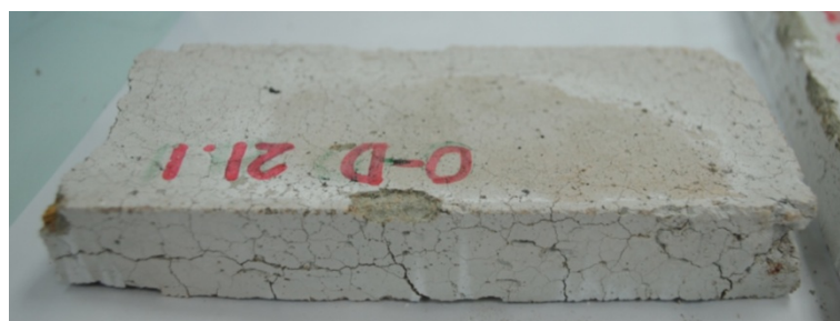
Fig. 4 – 14 Deterioration of oven – dried condition specimen 21.1 mm thick
