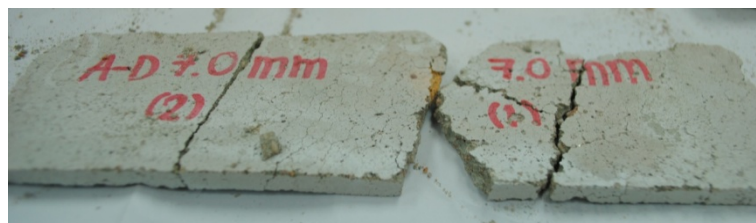
Fig. 4 – 4 Deterioration of air – dried condition specimen 7.0 mm thick
