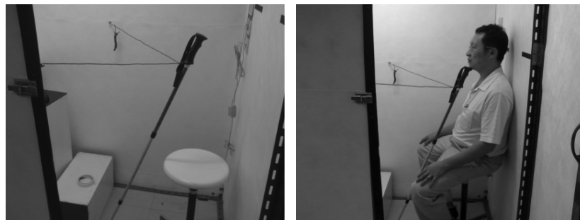
Figure 4-5 Chin rest (left) and demo (right) for controlling the correct viewing distance.
