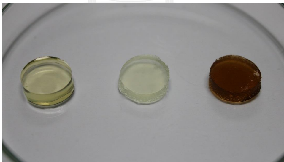
Figure 4.1 As-prepared hydrogels Left: neat gelatin, middle: gelatin/PVA, and right: gelatin/PVA with AgNO 3 .
