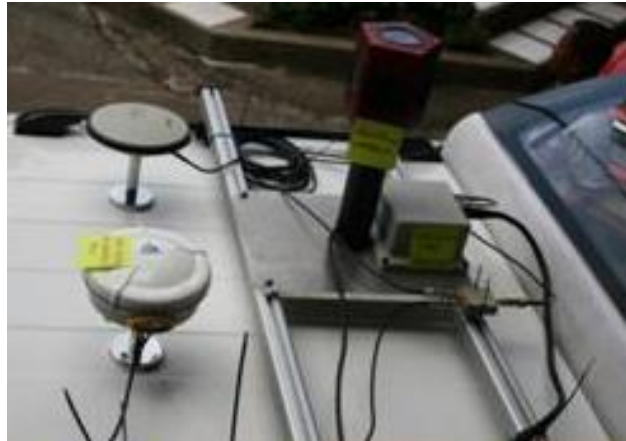
Figure 4.6 Instruments attached to the rooftop of a car. The Trimble R8 used as the rover for this study is shown in the lower left.
