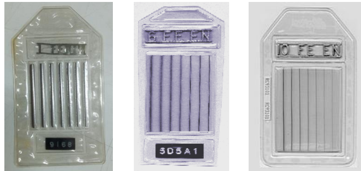
Figure 2.24 Wire DIN IQI according to EN 462-1 (and ISO 19232-1) each size composes of 7 wires, place parallel 5 mm distance from each other [8]
