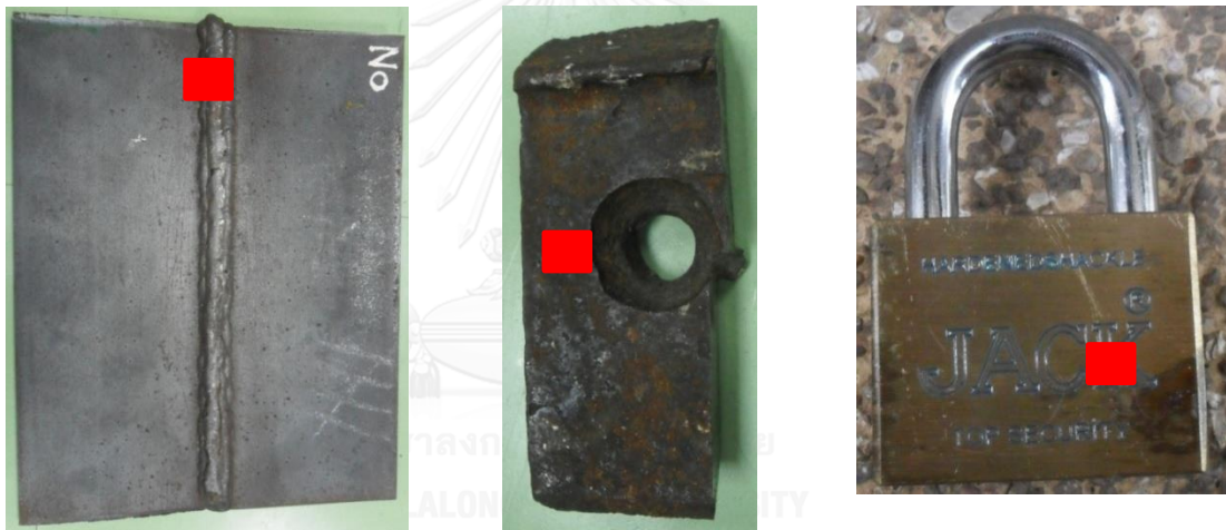
Figure 3.24 Showing the positions on the test specimens where the transmitted gamma-rays were measured with the developed device (These positions were expected to have the OD of 2.0 on the radiographs)
