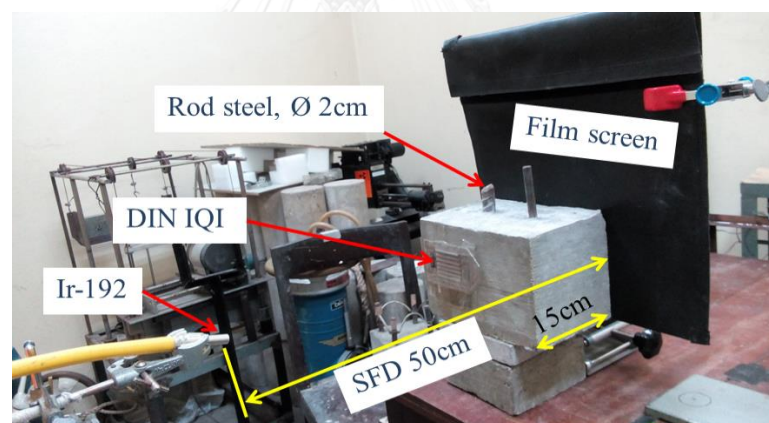
Figure 3.13 Experimental setup for investigates the image sensitivity from steel rod inside the concrete block specimen
