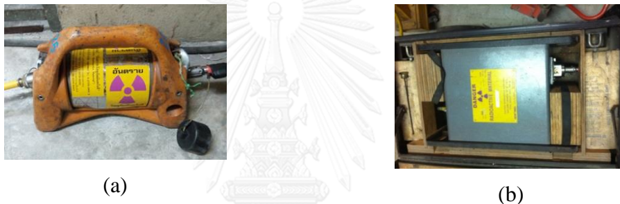
Figure 2.11 Shielding of radioactive source for Ir-192 (a), for Co-60 (b)
