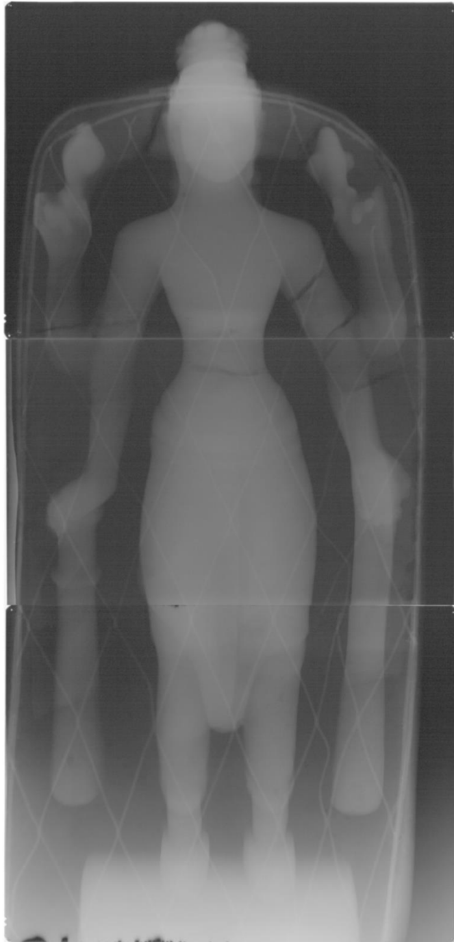
Figure 4.34 Radiograph of the Narayana statue using the lead screen-film technique taken with Ir-192 source
