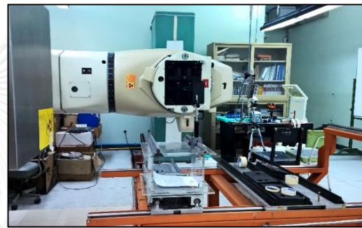
Figure 35. ^{60}\text{Co} source in teletherapy machine at the DMSc
