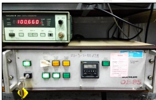
Figure 32. The control unit for ^{137}\text{Cs} source
