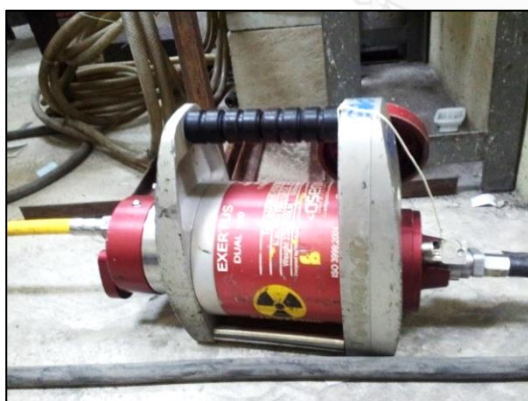
Figure 18. The ^{192}\text{Ir} source in the shielded container from NDT, Thailand
