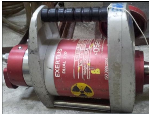
Figure 4. ^{192}\text{Ir} source in shielded container
