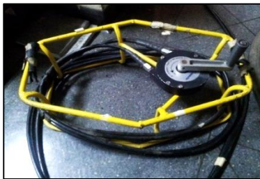
Figure 27. The use of wind-out to bring ^{192}\text{Ir} from the shielded container to the edge of projection tube
