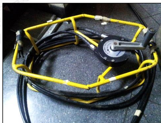
Figure 17. Wind-out which was used to bring the ^{192}\text{Ir} from the shielded container
