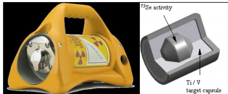
Figure 5. ^{75}\text{Se} source in shielded container and the structure of capsule of ^{75}\text{Se} . Source: www.ndt.net
