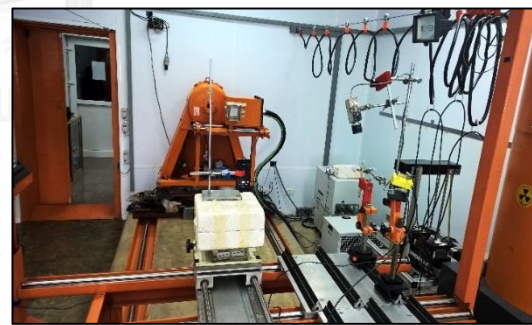
Figure 33. ^{137}\text{Cs} source in lead shielding at the OAP
