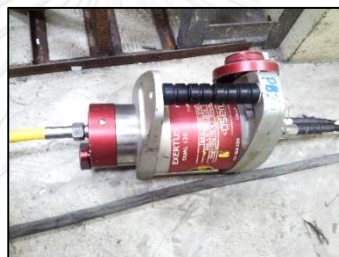
Figure 29. ^{192}\text{Ir} source in the shielded container
