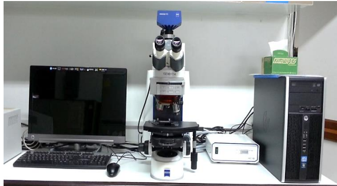
Figure 15 The photomicroscope (Zeiss Image A.2 Axio, Germany) with an attached digital camera (Cannon Power shot A640, Japan)
