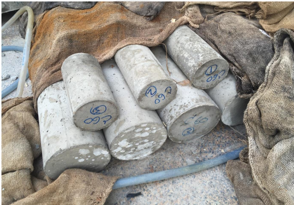
Figure 3.2-5 Wet cure and storage of cylinders
