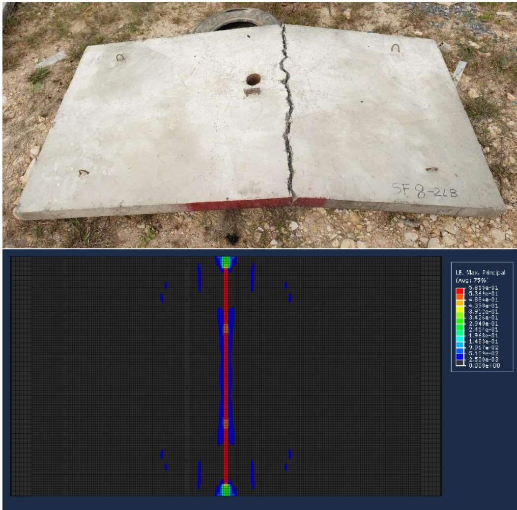
Figure 5.2.3- 1 Crack propagation at the bottom surface of panel 60SF2LB
