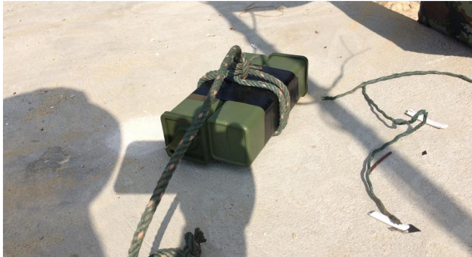
Figure 3.1-7 Two of 1lb TNT explosive tied together to form a 2lb loading
