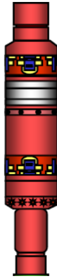
Figure 3.2 Typical hydraulic set retrievable packer without hold down buttons which represent PHL/HS type
