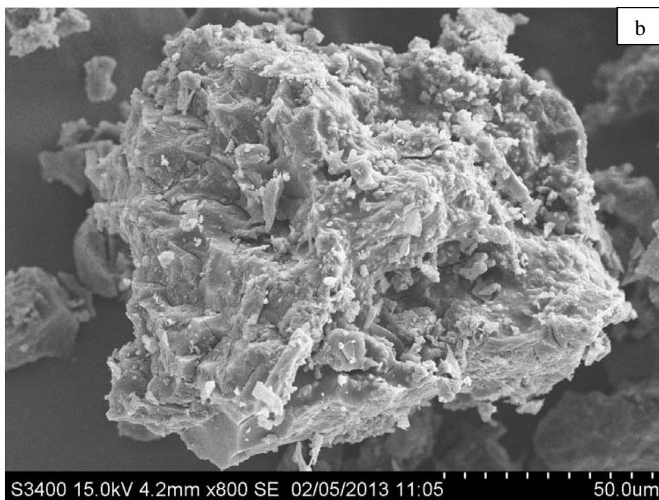
Figure 5.9 SEM micrographs of aluminium (12 wt%) modification avicel supported nickel (20 wt%) catalyst, Ni/AV: (a) 20 wt% Ni/AV-12Al (scale 10 \mu\text{m} ), (b) 20 wt% Ni/AV-12Al (scale 50 \mu\text{m} )
