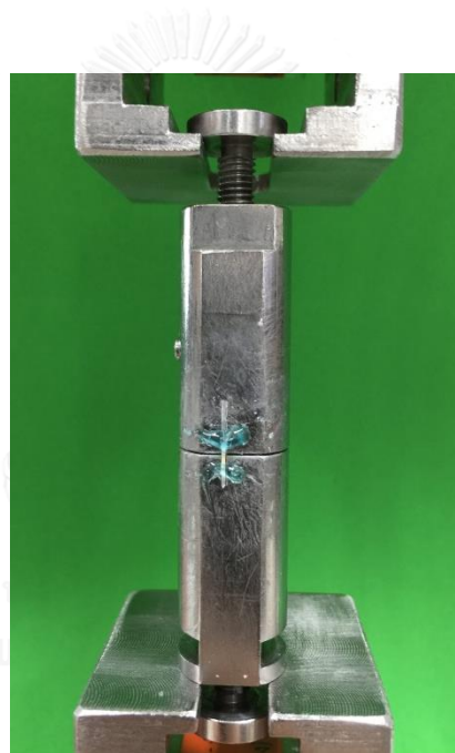
Figure 11 Attached specimen on the universal testing machine (EZ-S, Shimadzu, Japan)
