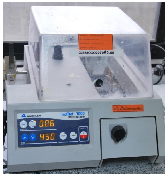
Figure 8 Slow-speed diamond saw; Isomet™ 1000 Precision Saw, Buehler, USA
