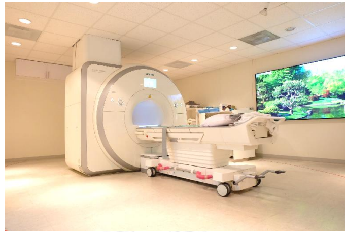
Figure 3.6 MRI 1.5 Tesla (MAGNETOM Aera; Siemens AG, Erlangen, Germany).
