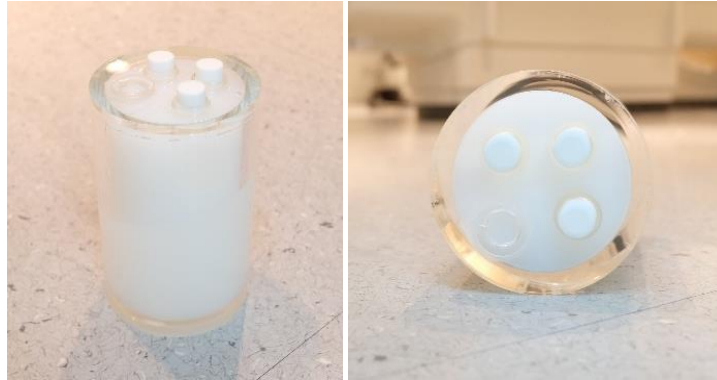
Figure 3.10 PVA-gel phantom (NIKKO FINES INDUSTRIES Co.,Ltd, Tokyo, Japan).
