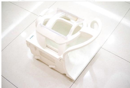
Figure 3.7 The 20-channel head/neck phase array coil.
