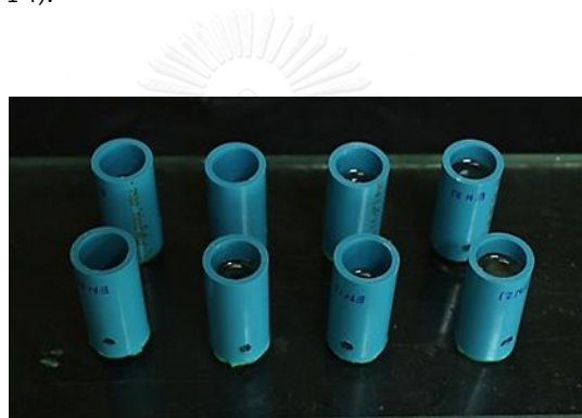
Figure 13 Denture teeth embedded in auto-polymerized PMMA.
