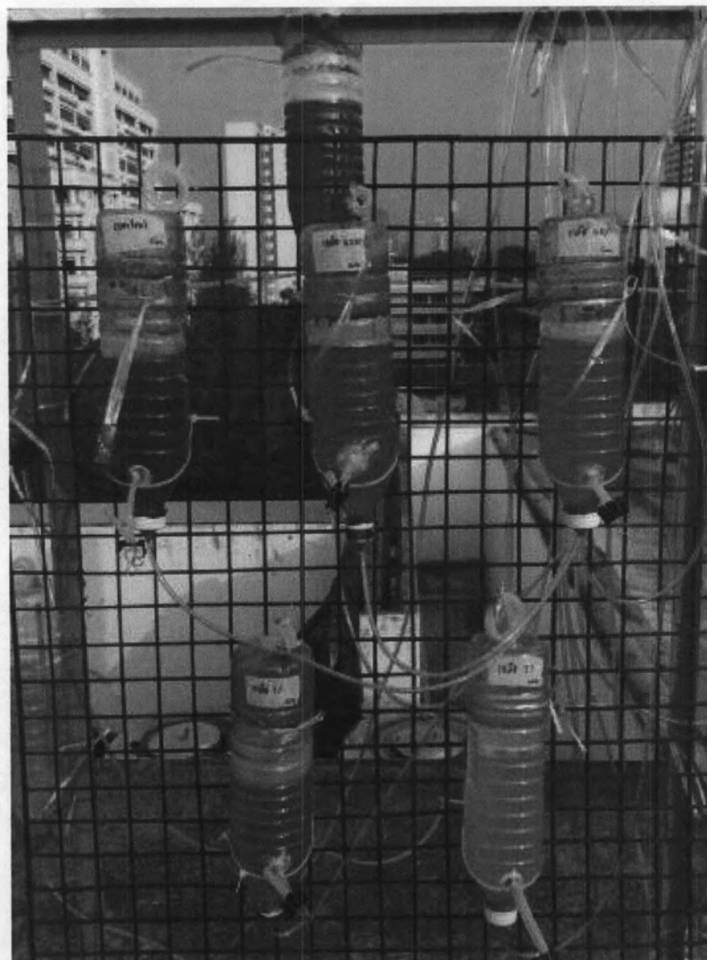
Figure 3.1 Astaxanthin production in 1.5L bubble column photobioreactor (Outdoor experiments)
