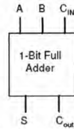
Figure 2: One-bit Full Adder
