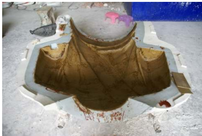
Figure 78 Stick wax sheet on the adhesive solution.
