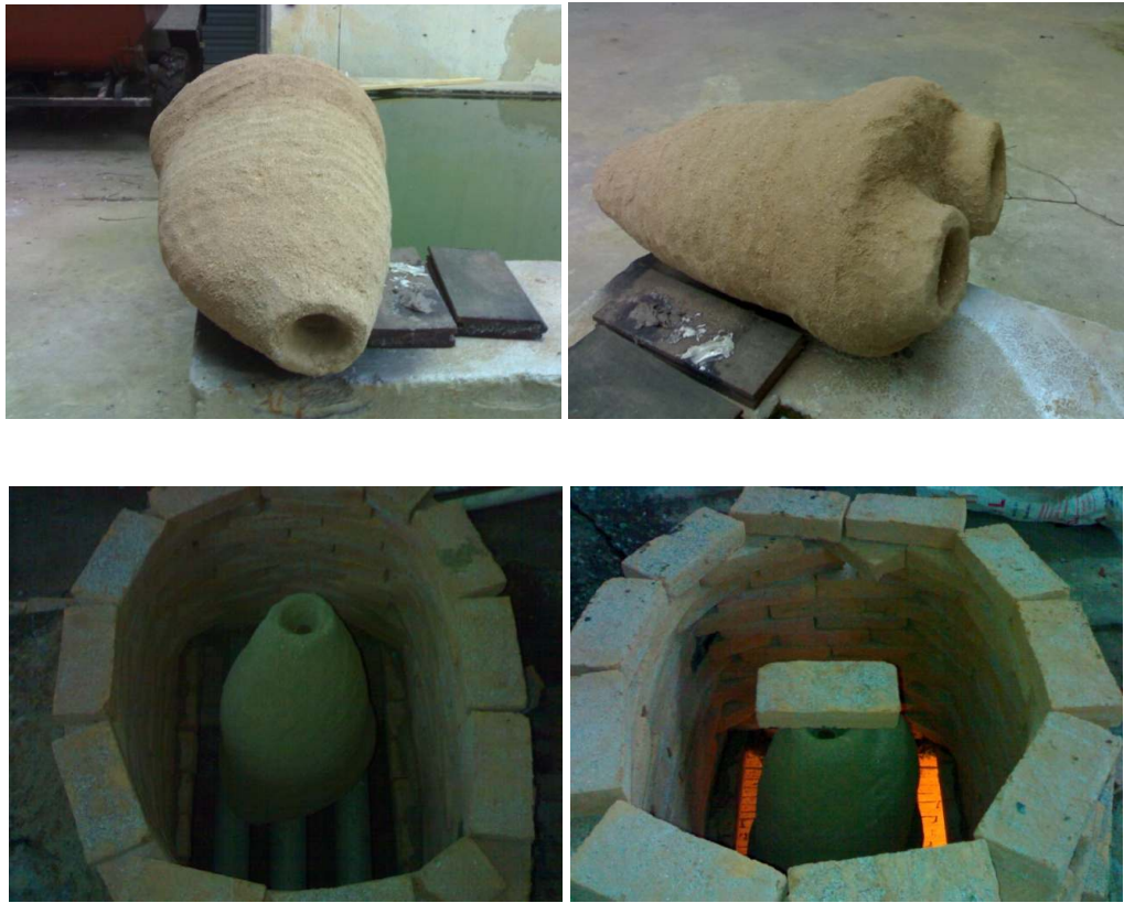
Figure176 Dry mould placed in the kiln and covers the hole on the mould with brick.
