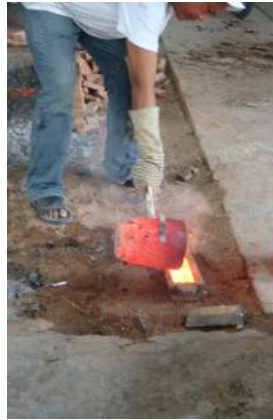
Figure 202 Pouring remaining bronze in the ingot pot.
