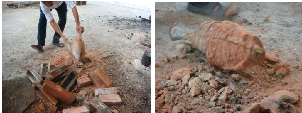
Figure 205 Breaking the mould revealing the layers of burnt clay and sand plaster.
