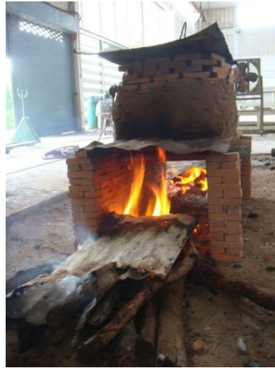
Figure180 Giving heat under the mould from fire burning at the two mouth of the kiln.
