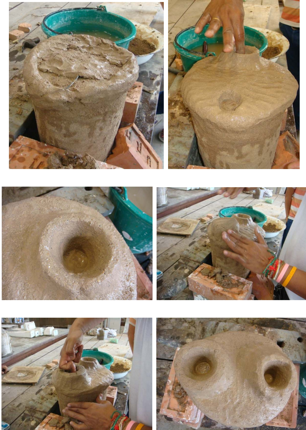
Figure169 Make air vent and pouring cup with clay and sand plaster.
