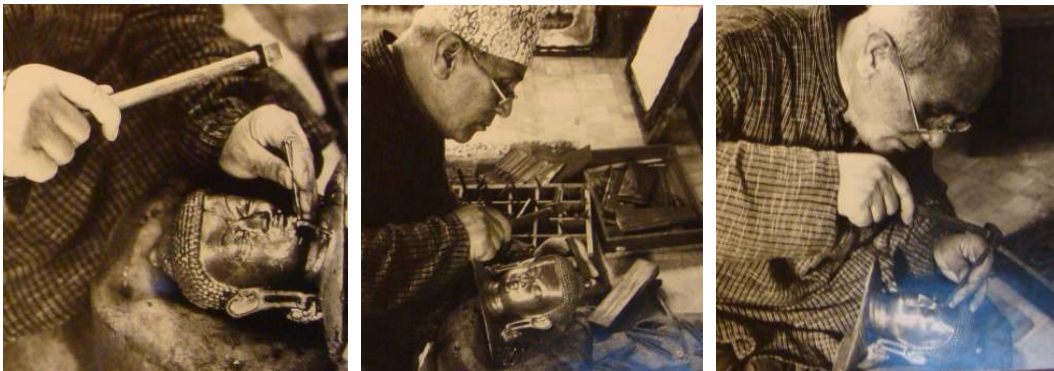
Figure 215 Cutting off channels and hammering for refinement
