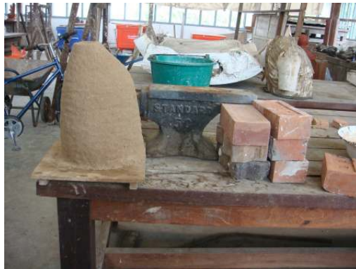
Figure 165 Making inspection hole on the exposed wax rod which will be covered by brick while melting wax out.
