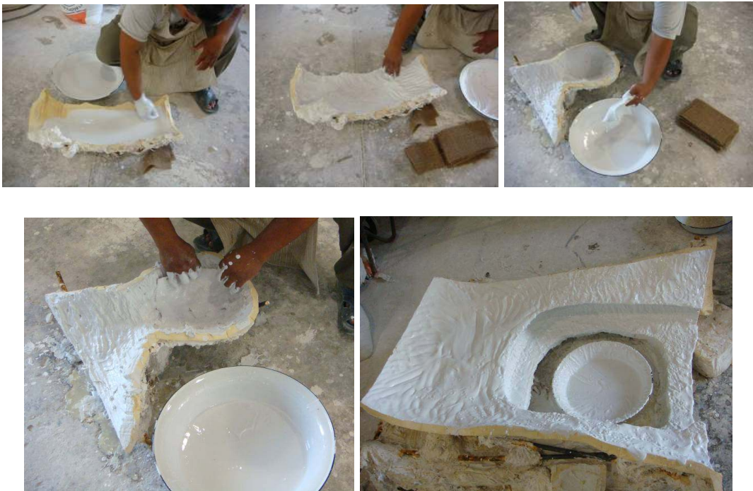
Figure 57 Applying jute fabric mixed plaster.
