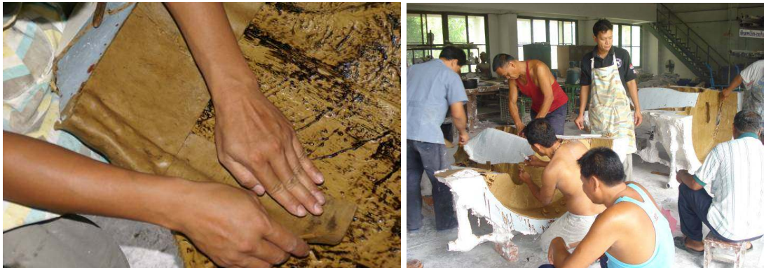
Figure 77 Apply adhesive solutions on the second layer of wax.
