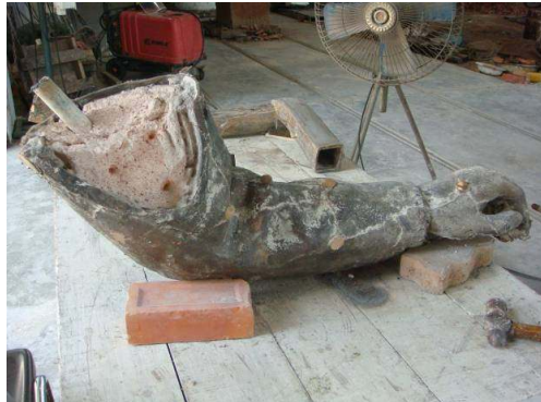
Figure 107 Cut off the bronze channels and runners.
