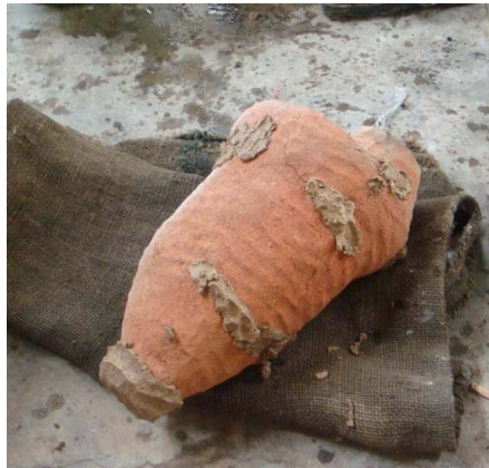
Figure196 Carefully taking out the hot mould from the kiln and place on the ground.
