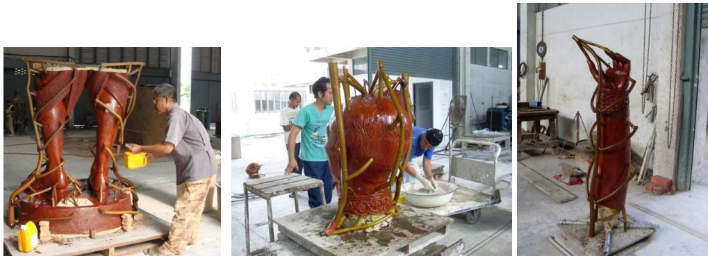
Figure 85 Applying methyl alcohol on the wax sculpture.
