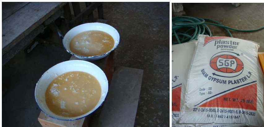
Figure 37 Gypsum Plaster mixed with water and color.
