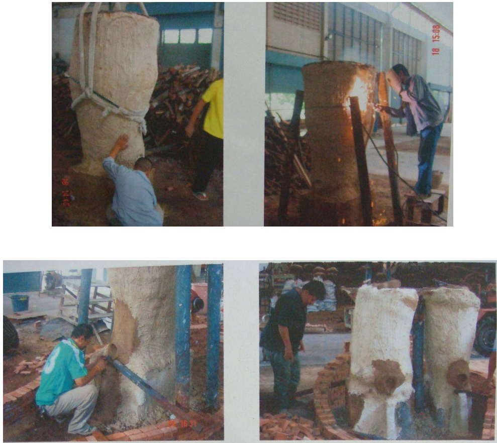
Figure 89 Prepare mould and kiln for melt wax.
