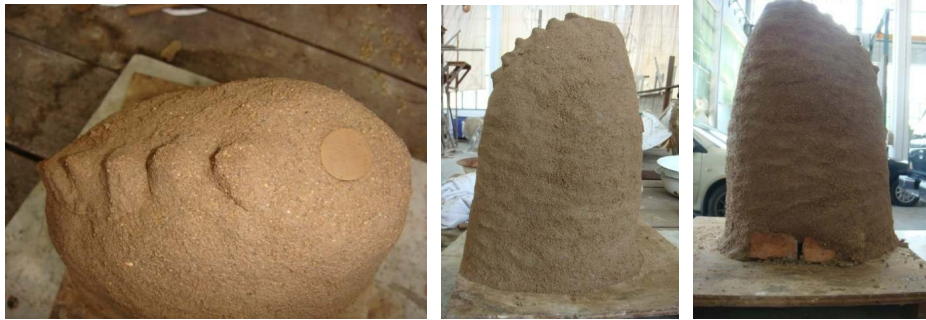
Figure 160 Wax channel exposed and finished second layer of clay and mud plaster.
