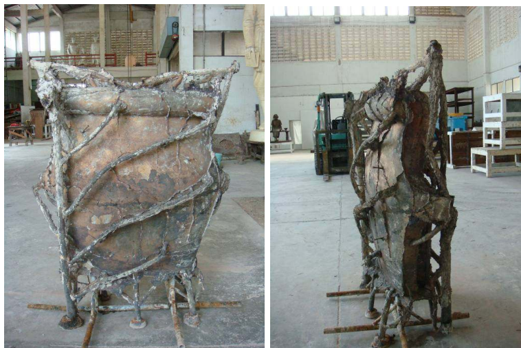
Figure 106 Bronze layer on the place of wax layer.
