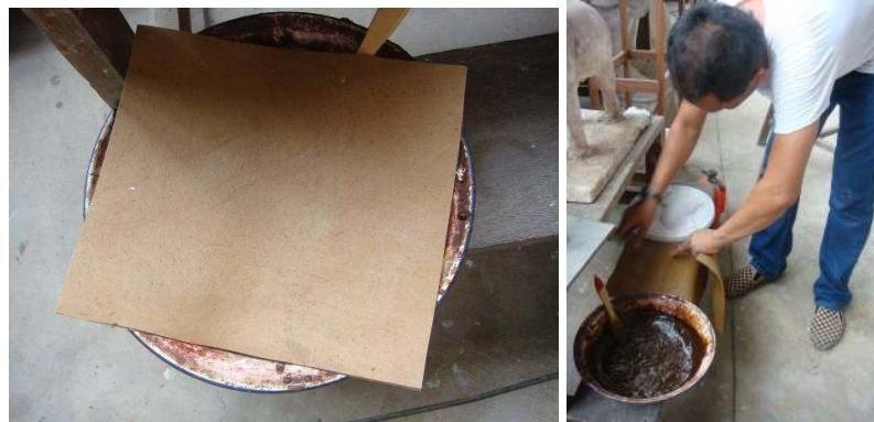
Figure 131 Wax sheet make warm and cut into required size.
