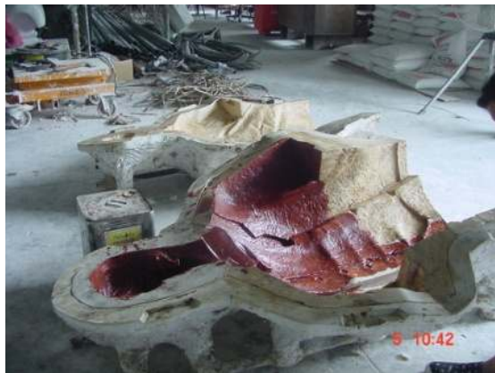
Figure 74 Apply first layer of liquid wax on the silicon.
