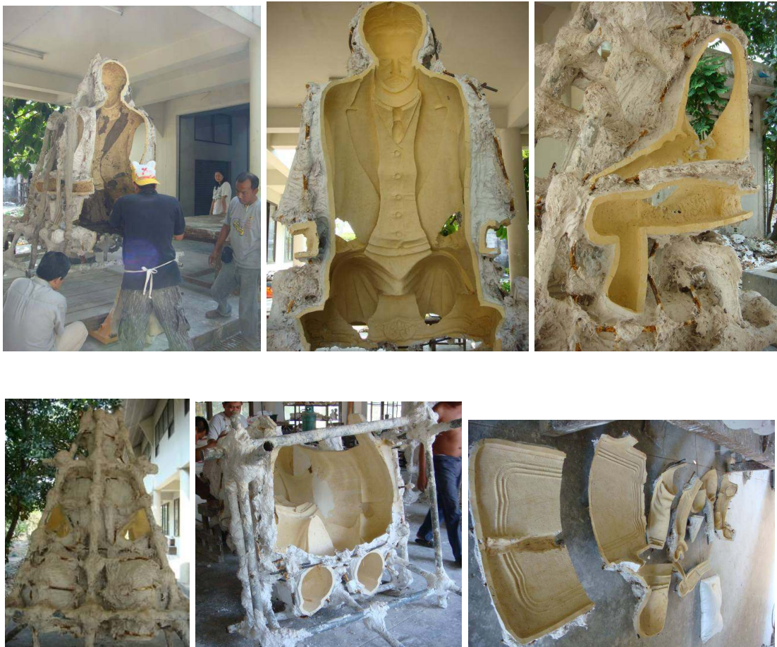
Figure 53 Clean the plaster mould with water spray.
