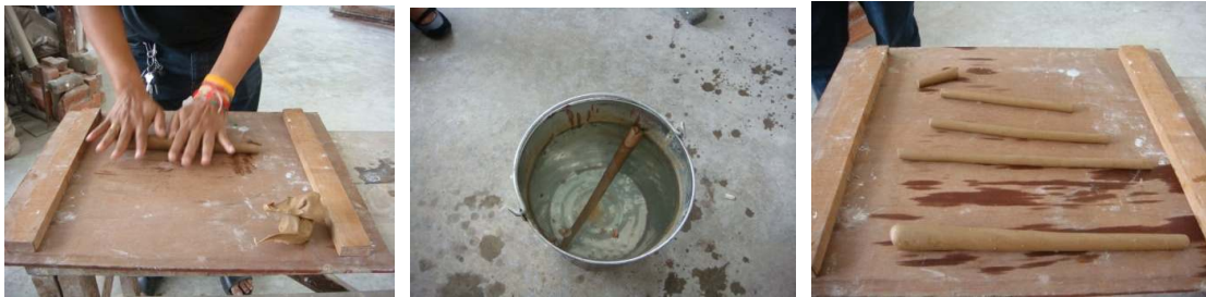
Figure 145 Wax rolled on a wooden board to make conical and cylindrical wax rods.
