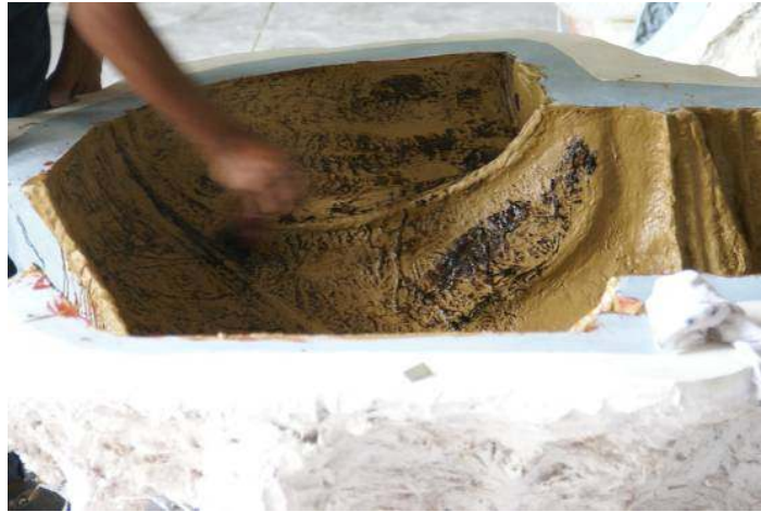
Figure 77 Apply adhesive solutions on the second layer of wax.
