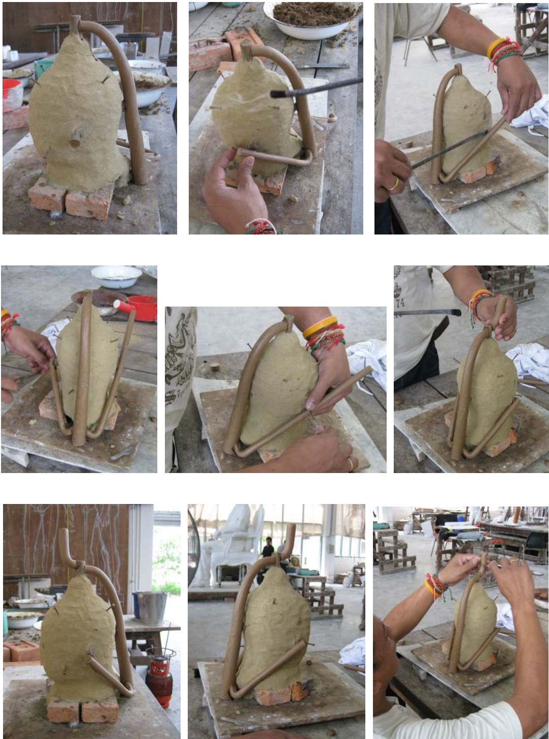
Figure 157 Attach wax channels and runners.
