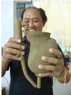
Figure 154 Showing how the wax rod as sprue is going to be attached before attaching the wax rods.
