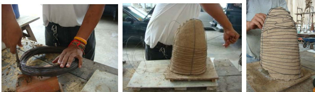
Figure162 Surround and tie iron wires around the mould.
