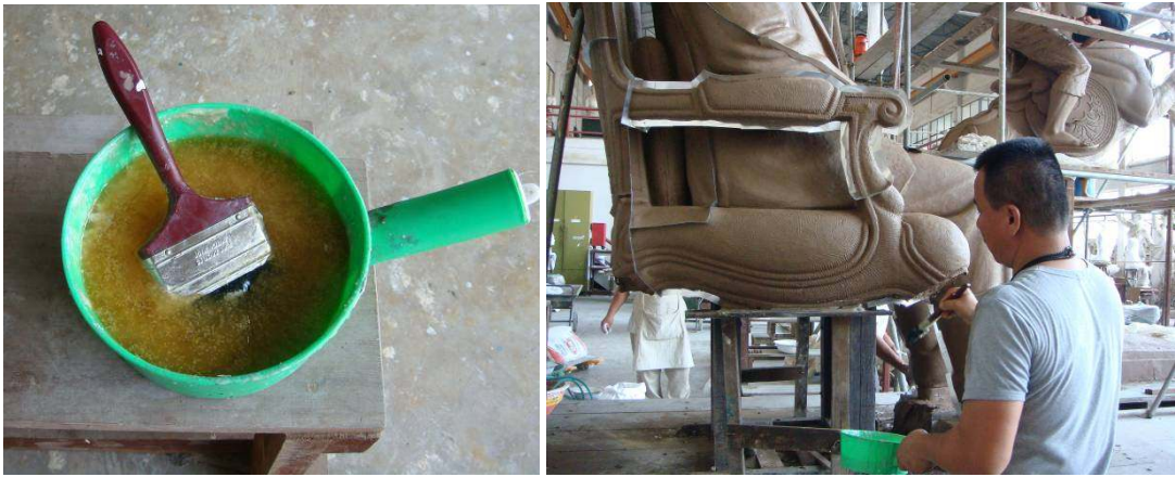
Figure 36 Mixture of Coconut oil and soap solution apply on the surrounding wooden surface.
