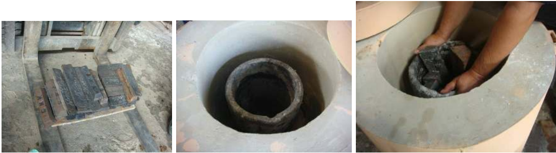
Figure 98 Bronze ingots placed in the crucible inside the gas furnace.
