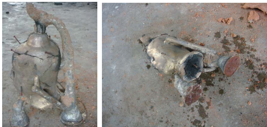
Figure 208a Bronze Buddha head with bronze channels and nails revealing.
