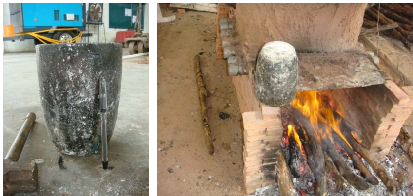
Figure184 Crucible and pre heat on the heat of fire.
