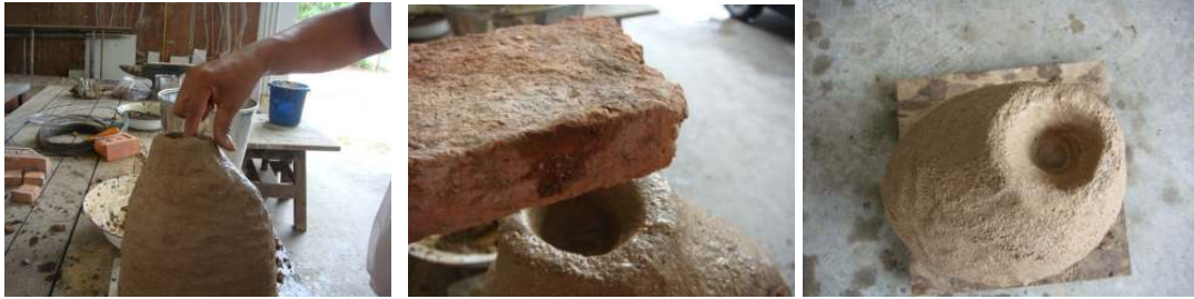
Figure 165 Making inspection hole on the exposed wax rod which will be covered by brick while melting wax out.
