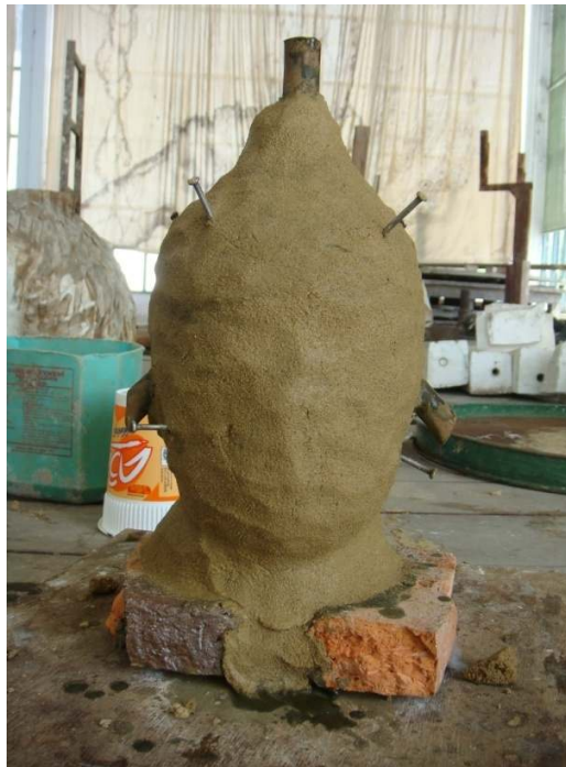
Figure 153 The clay mould covered sculpture.
