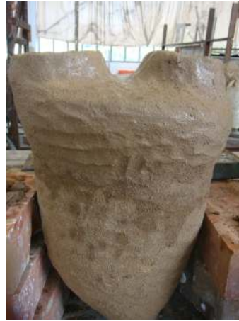
Figure170 The finalized mould left for dry.
