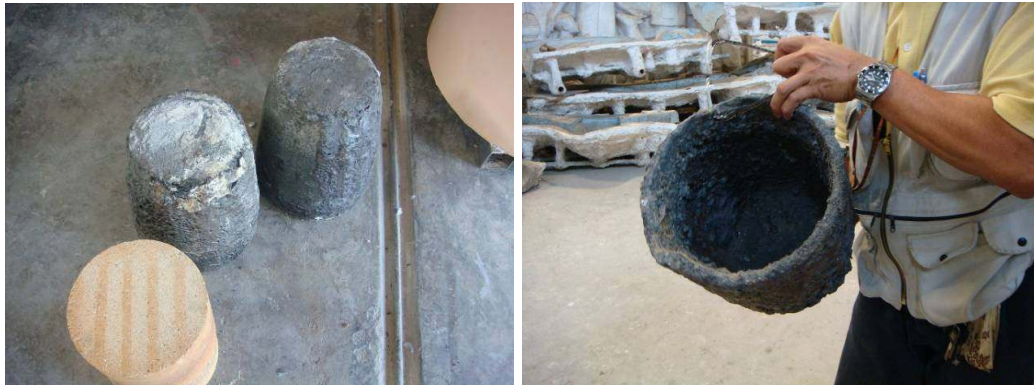
Figure 95 Rice husk tempered crucibles and cement stand for crucible.
