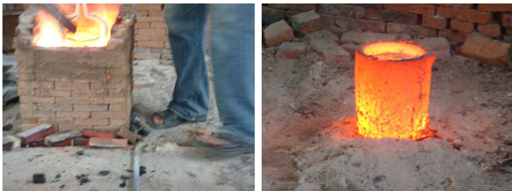
Figure199 Take out crucible from the furnace and place on ground.
