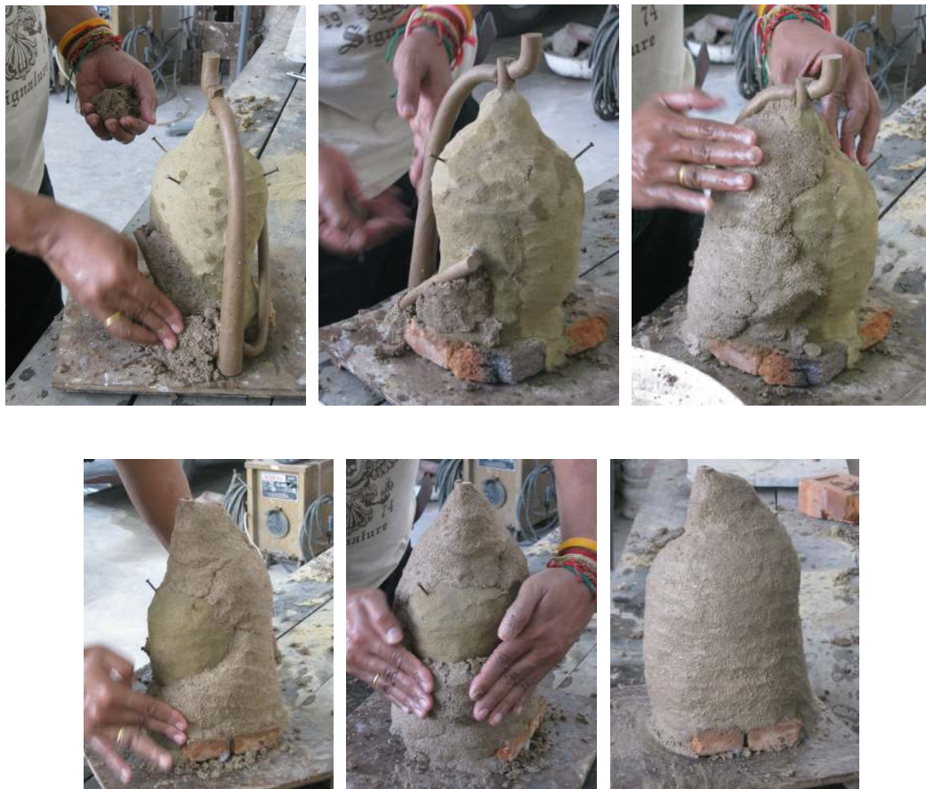
Figure 159. Apply second coat of sand mixed clay on the mould to cover wax rods and nails.
