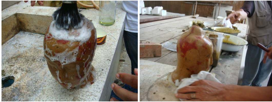
Figure 142 Wash the wax with soap water and dry with cloth.
