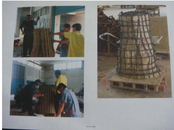
Figure 87 Strengthen wax mould with iron rods.
