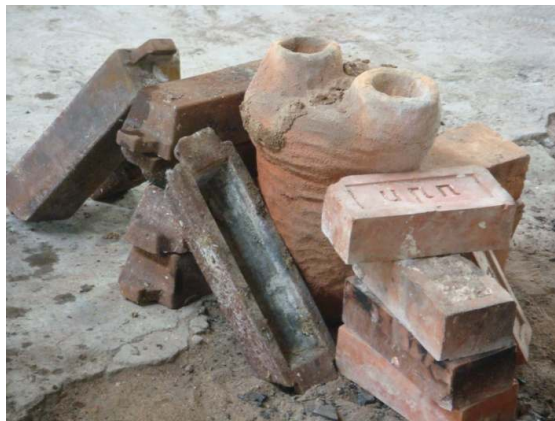
Figure197 Close cracks and the single hole with wet clay plaster and securely place upright with the two holes facing up.
