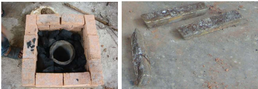
Figure193 Surround the crucible with big charcoal pieces and bronze ingots.
