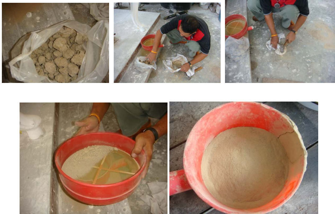
Figure 140 Strain soft clay dust.
