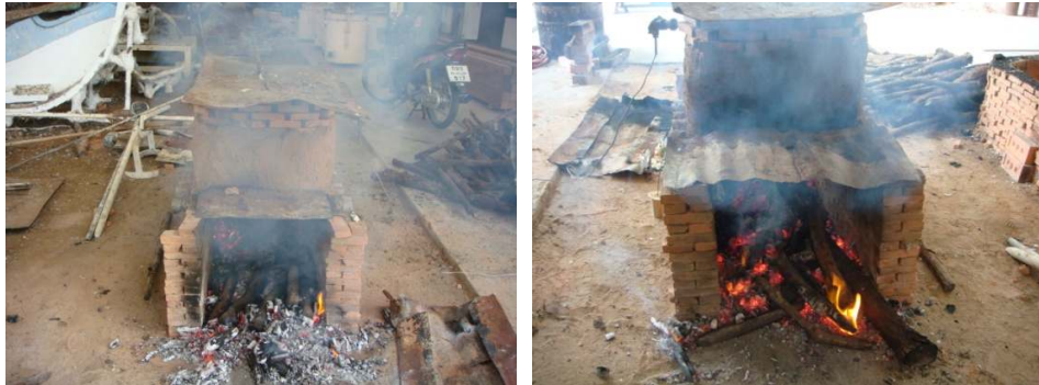
Figure182 After wax stops to melt give fire directly under the mould.
