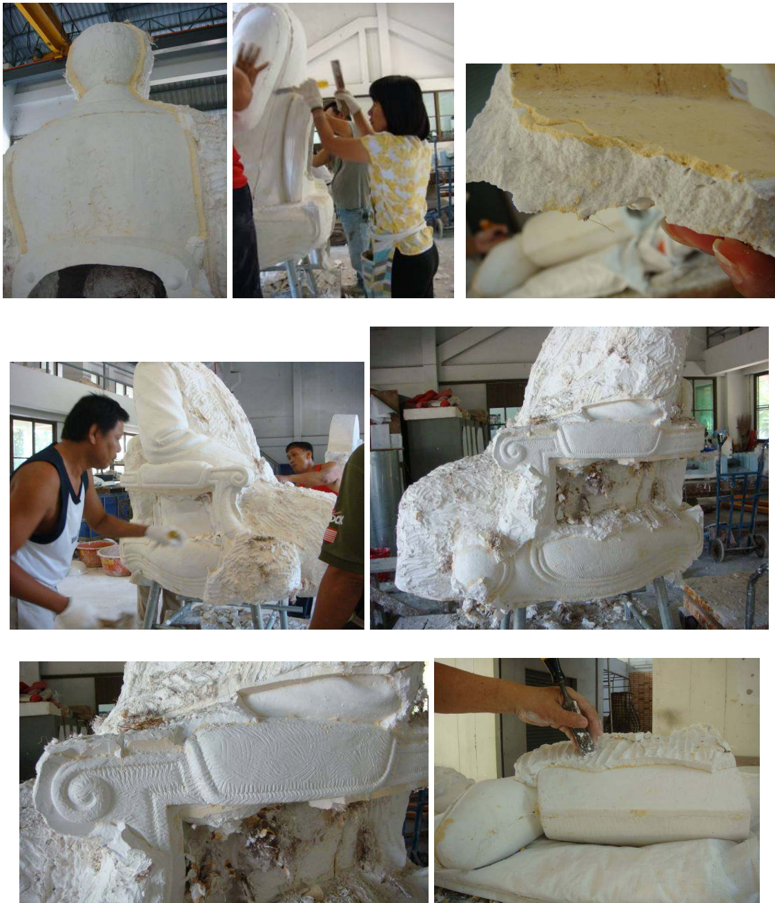
Figure 63 Break off the first layer of Gypsum plaster coat revealing the inner plaster mould.
