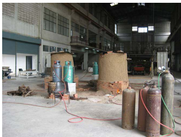
Figure 92 Gas cylinders on boiling water to make easy flow of gas
