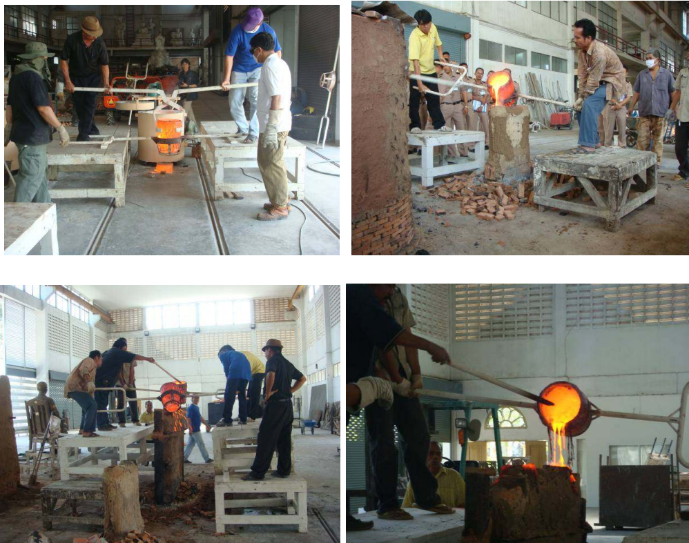
Figure 101 Pouring liquid bronze in the mould.
