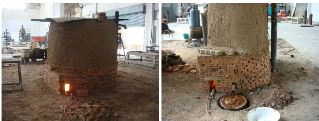
Figure 90 Brick Kiln to heat mould and melted wax flowing out.
