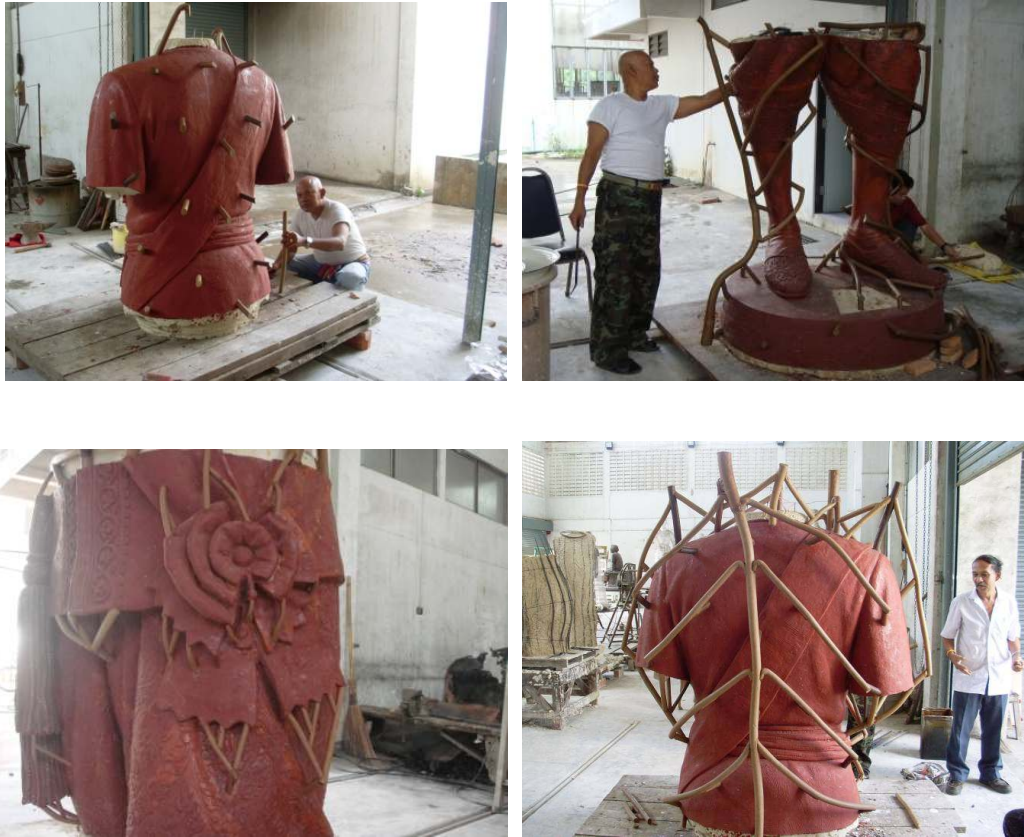
Figure 84 B Attach wax channels and runners.
