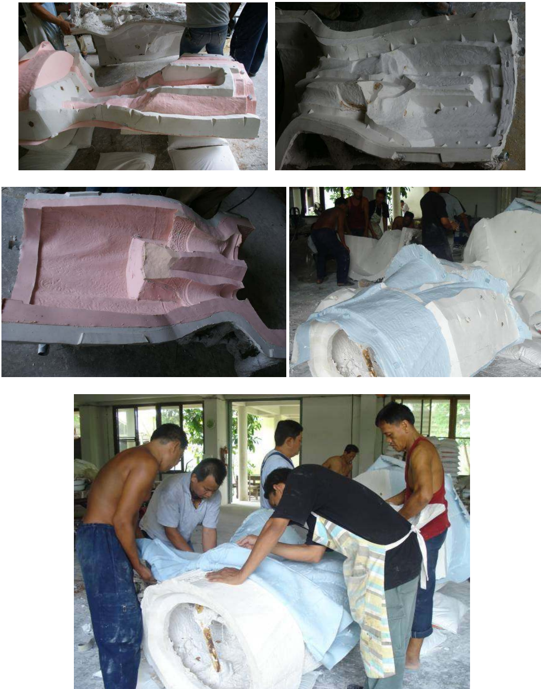
Figure 73 Take out Silicone rubber sheet from the plaster mould and insert on the outer plaster mould.
