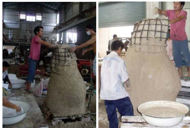
Figure 87 Strengthen wax mould with iron rods.
