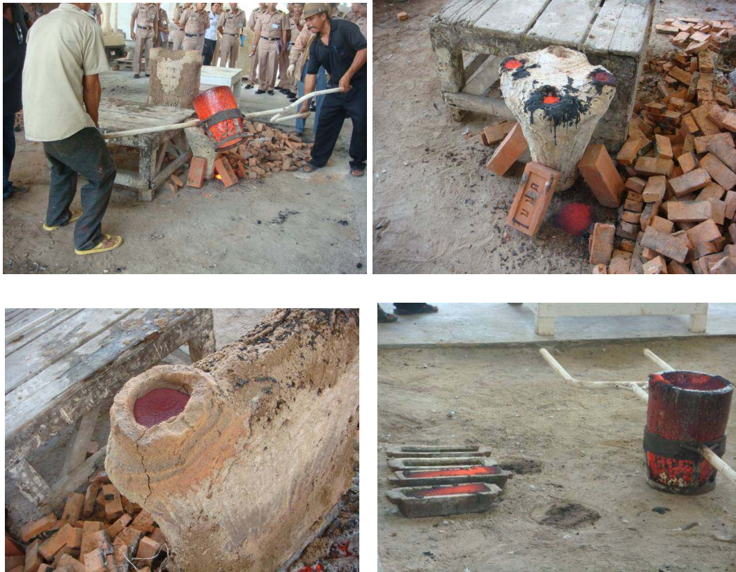
Figure 102 Liquid bronze seen in the pouring cup. Figure 103 Pour remaining bronze in ingot tray.
