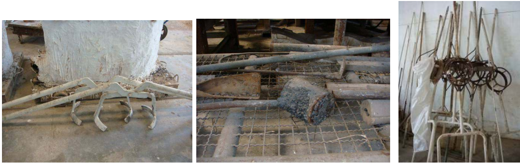
Figure 96 Different tools and utensils for casting bronze.
