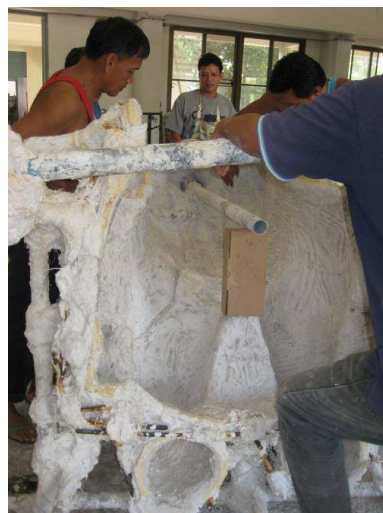
Figure 58 Strengthen the mould with zinc pipe.
