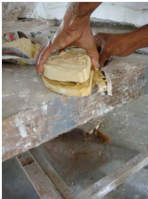
Figure 40 Taking out impression of the small piece.
