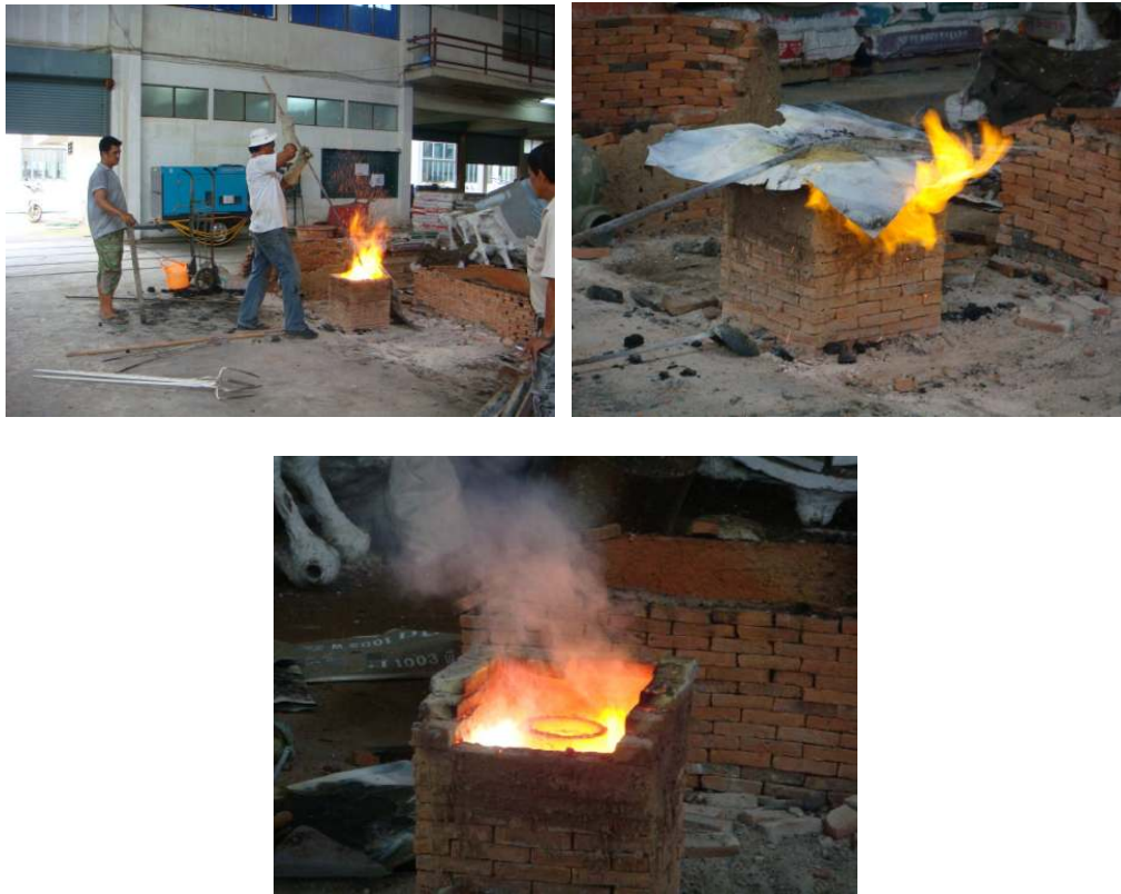
Figure198 Taking out impurities and raise air blow to prepare for pouring the melted bronze.
