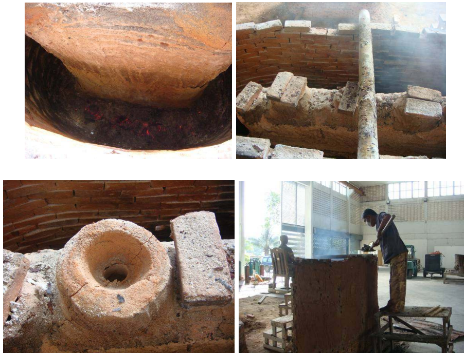
Figure 93 Pre heating the mould before casting bronze.
