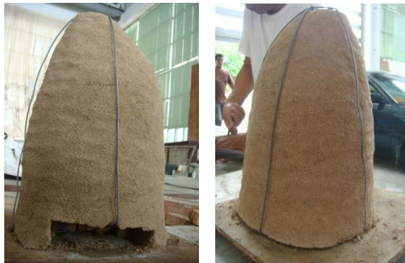
Figure 160 Wax channel exposed and finished second layer of clay and mud plaster.
