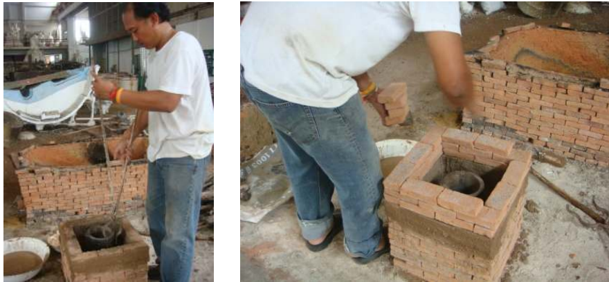
Figure192 Secure the crucible at the center and raise the furnace height by adding brick layer.
