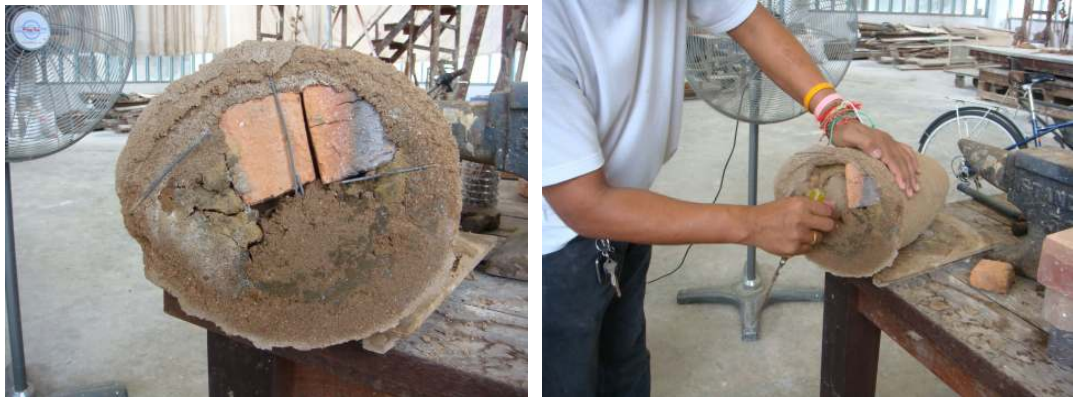
Figure166 Taking out brick bats from the base of the mould.
