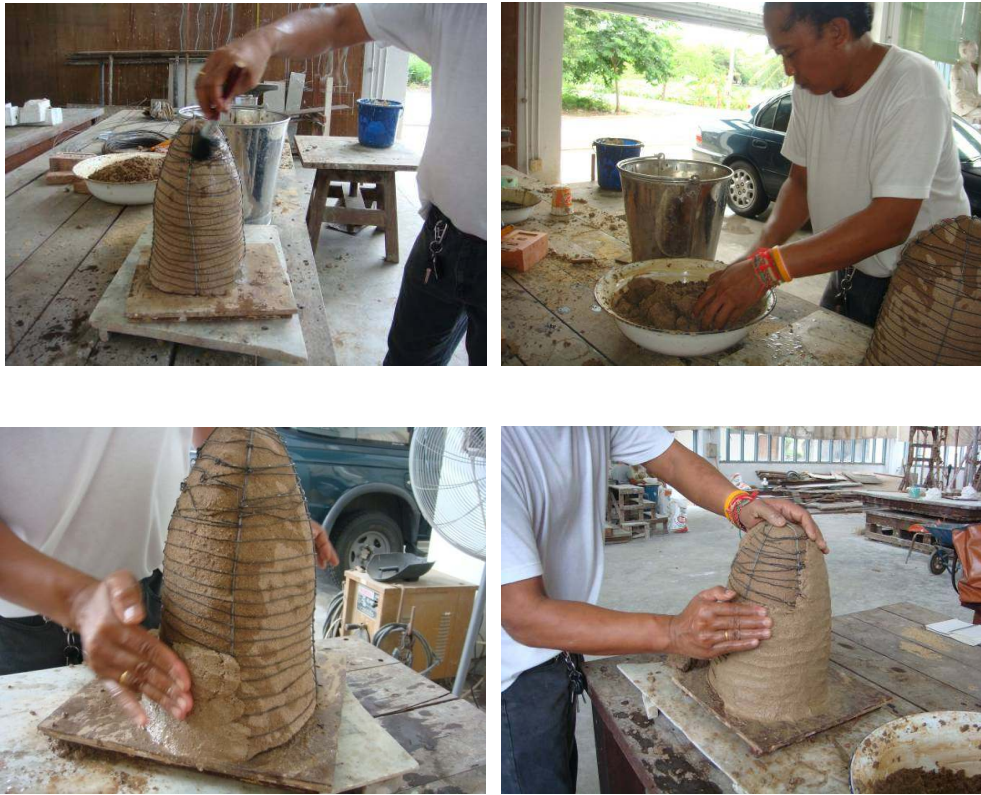
Figure163 Applying sand and clay mixed plaster on the iron wire.
