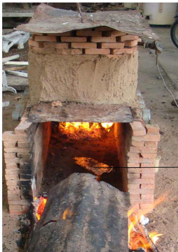
Figure181. Wax melting down from the mould.
