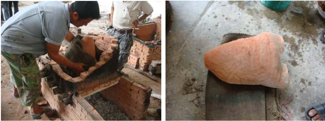
Figure196 Carefully taking out the hot mould from the kiln and place on the ground.
