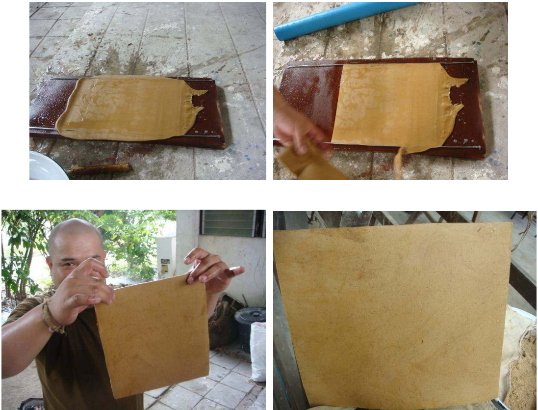
Figure 129 Wax sheets cut in square shape.
