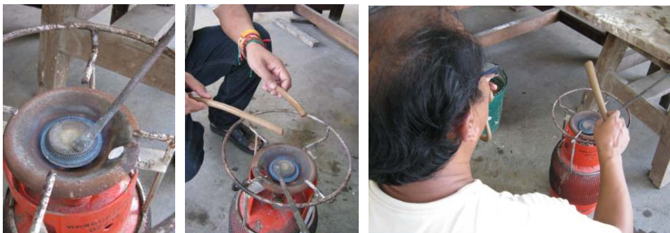
Figure 155 Heating iron and wax rods
