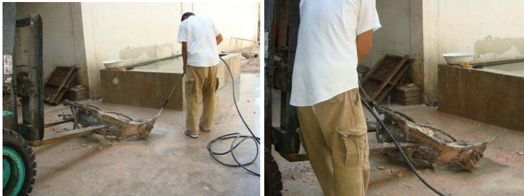
Figure 105 Clean inner and outer plaster with water jet spray.
