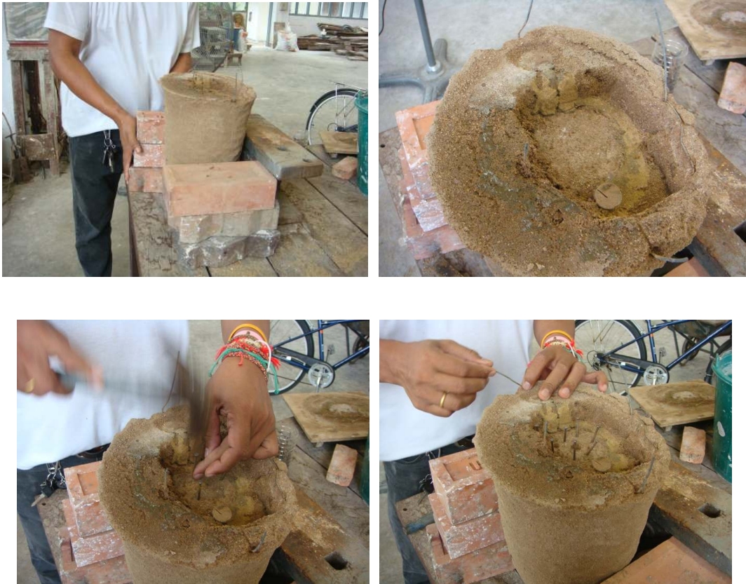
Figure167 Exposed wax rods and inserting the nails on the base of the core.
