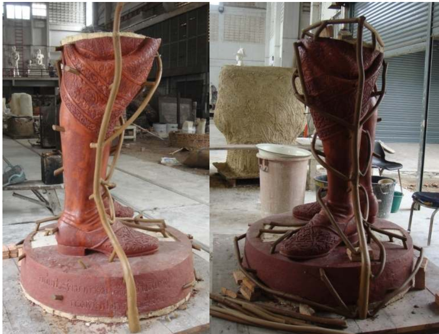
Figure 84 A Attach wax channels and runners.
