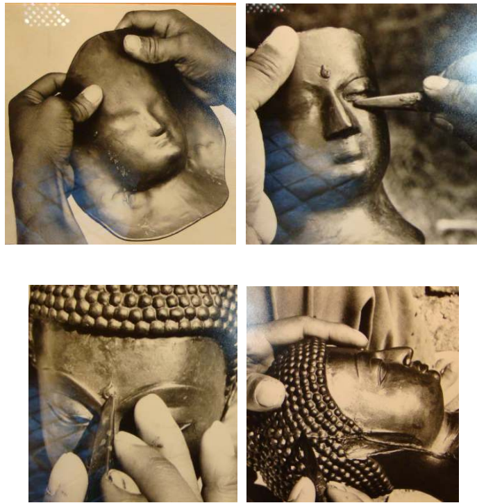
Figure 209 Shapping and joining the wax model of the sculpture.
