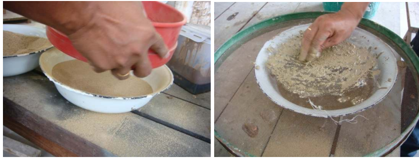
Figure 150 Strain sand and clay to get finer material.
