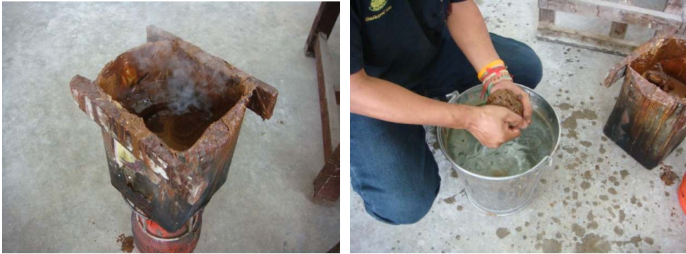
Figure 144 Melt wax and pour in cold water and kneaded by hand to make soft.
