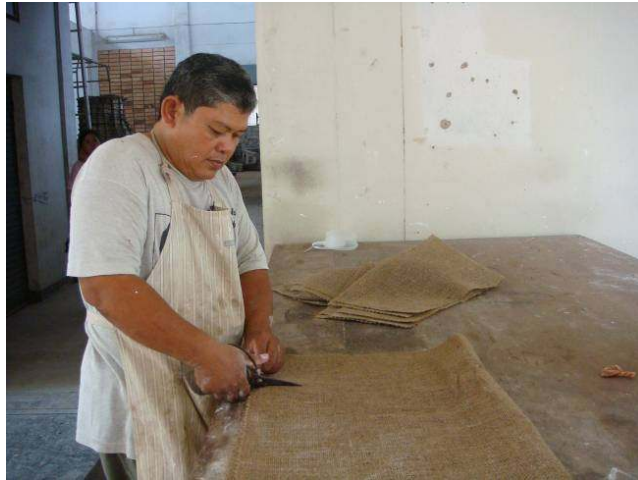
Figure 56 Cutting Jute fabrics to small pieces.
