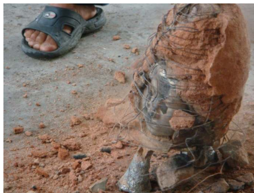
Figure 206 Revealing the bronze figure from inside the mould.
