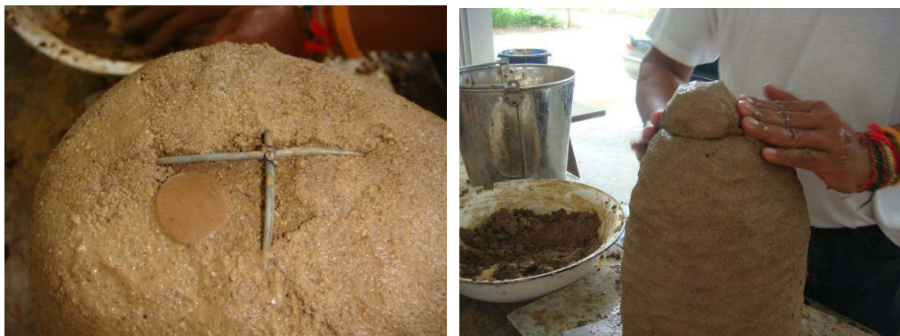
Figure164 Exposed wax rod and preparing to make cup on the wax rod.
