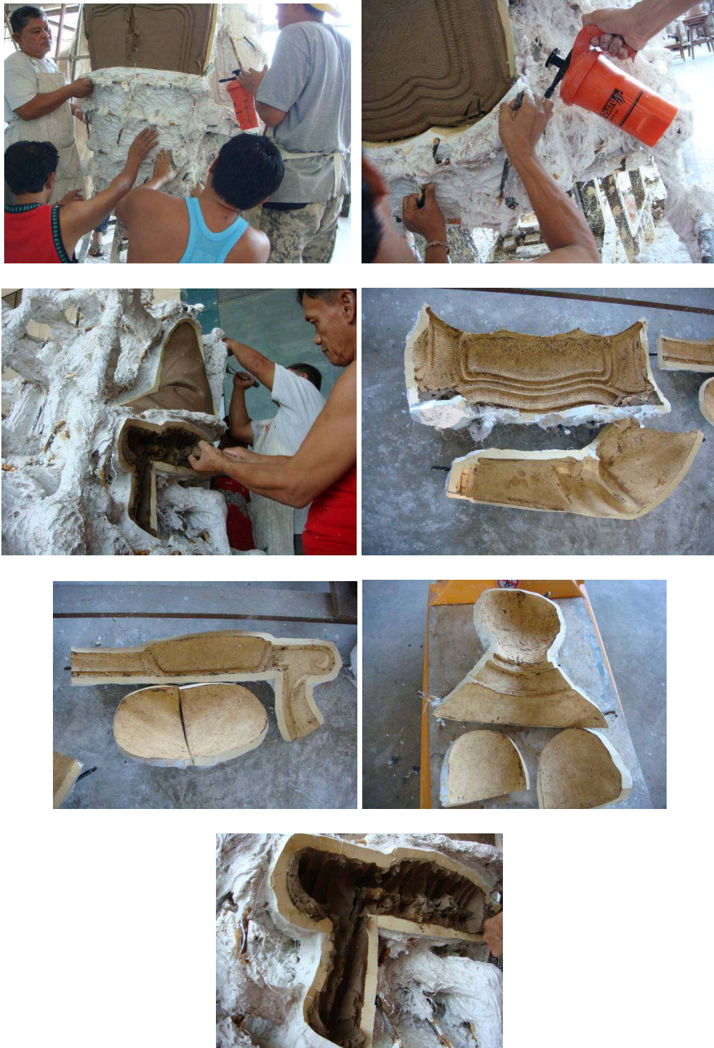
Figure 47 Separate plaster mould from the statue.
