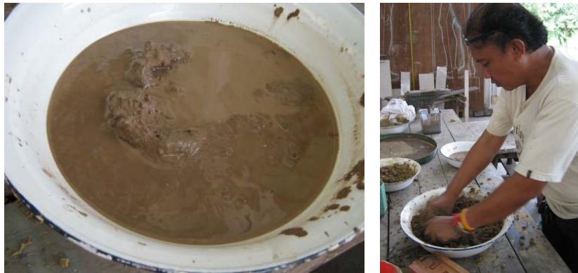
Figure 158. Mix water based clay with sand.
