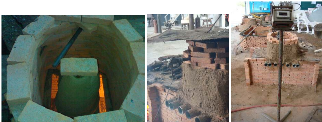
Figure177 Insert temperature measure rod in the kiln.
