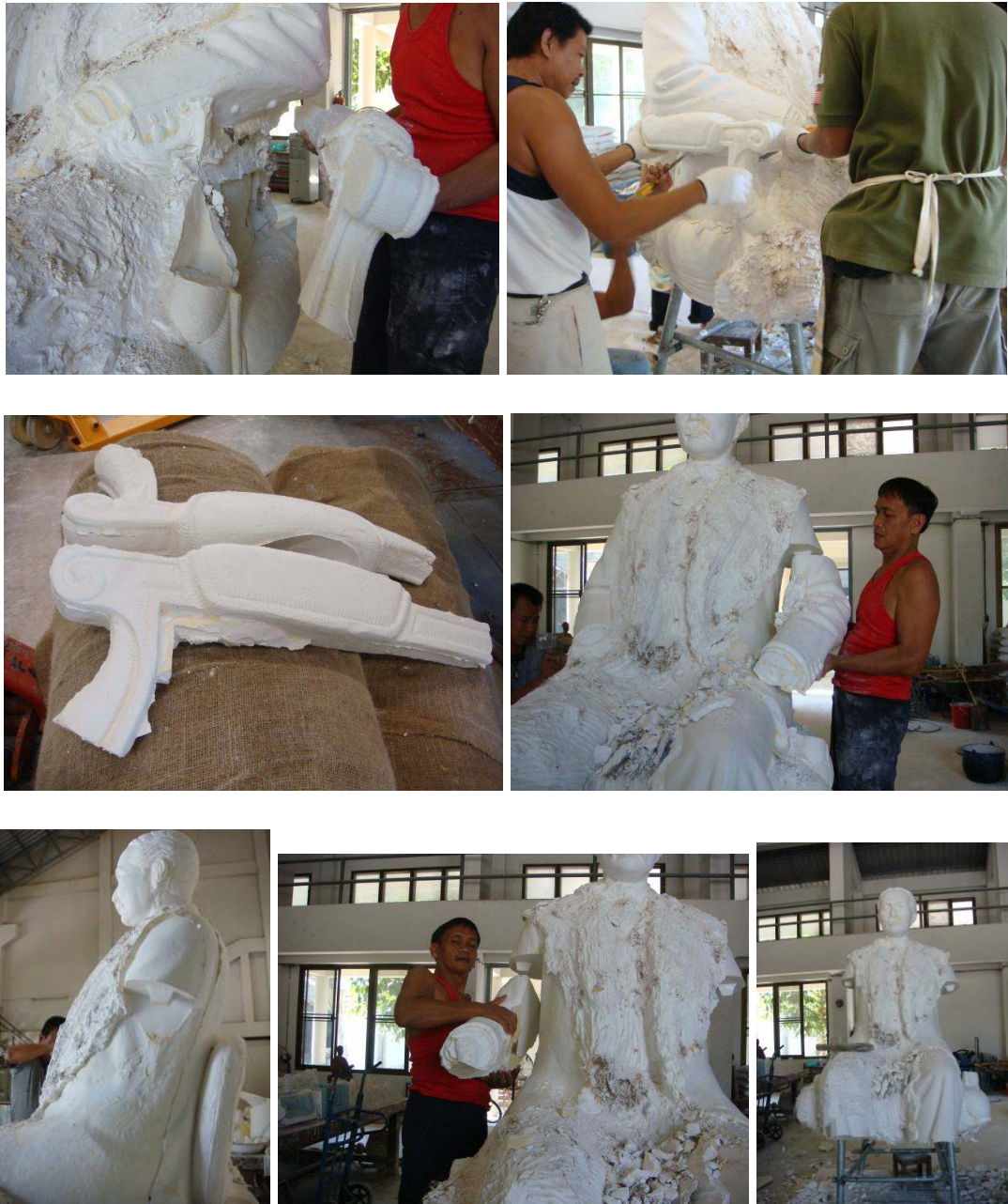
Figure 64a Detach parts of imprinted plaster mould from the main body.
