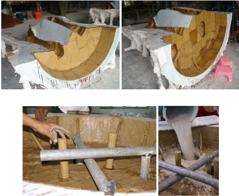
Figure 79 Join the two pieces together and strengthen the hollow with pipes and pour plaster and sand mixed liquid.
