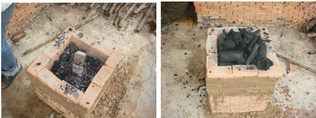
Figure194 Bronze ingots placed in the crucible and cover with burnt charcoal.
