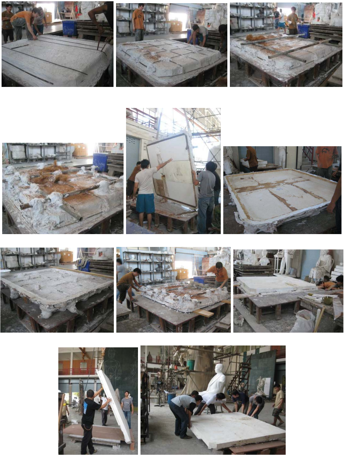
Figure 65 Making pedestal for statue.
