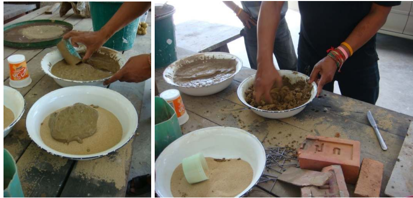
Figure 151 Mix sand and clay together.
