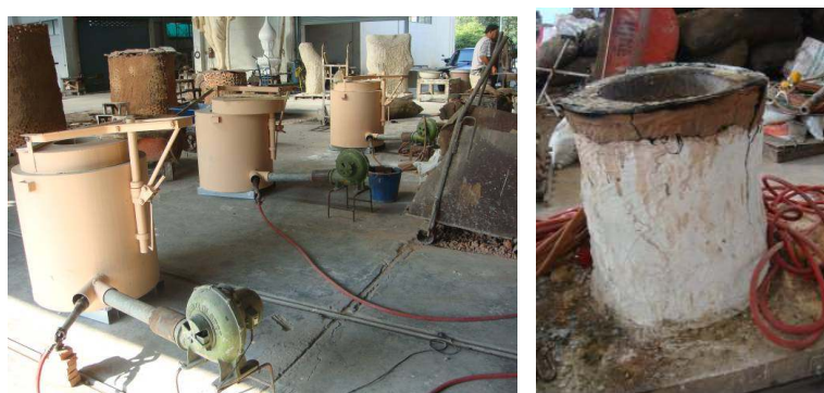
Figure 97 Modern gas furnace and traditional brick furnace for melting bronze.
