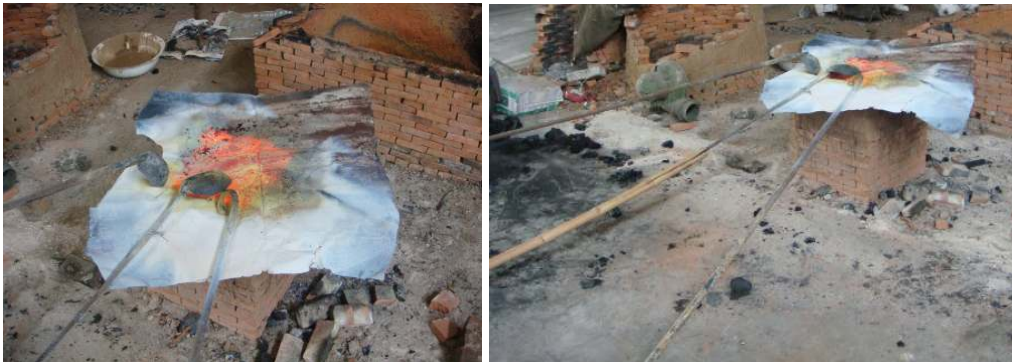
Figure195 Air blow makes the charcoal fire burn to its highest temperature.
