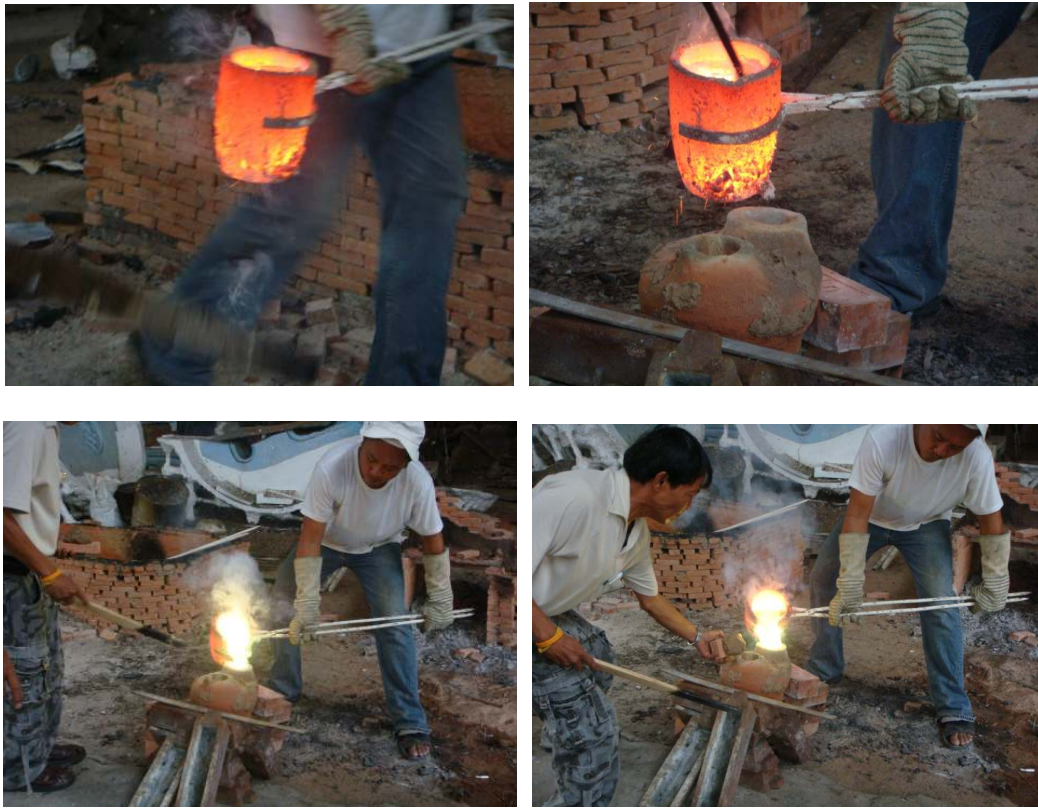
Figure 200 Hold up the crucible from the ground and pour molten bronze into the first hole.
