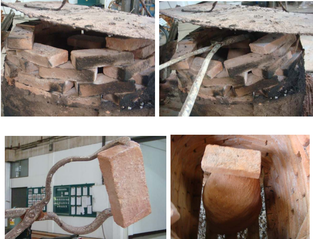
Figure185 Checking the brick placed on the upper hole of the mould.
