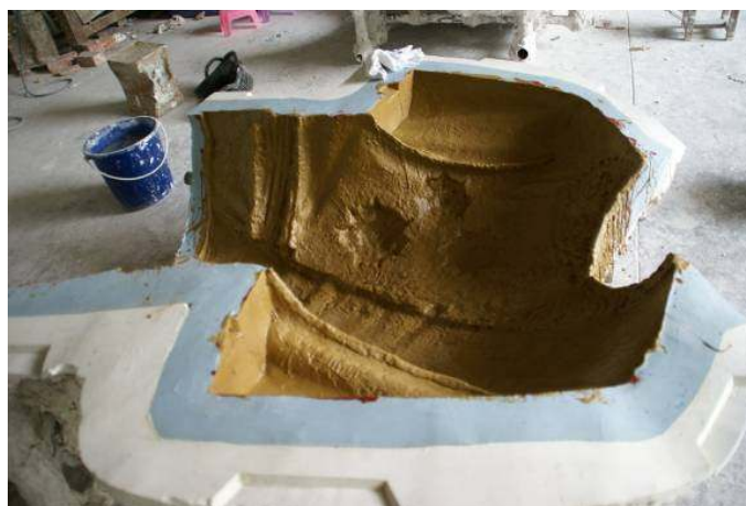
Figure 75 Apply second layer of melted wax.
