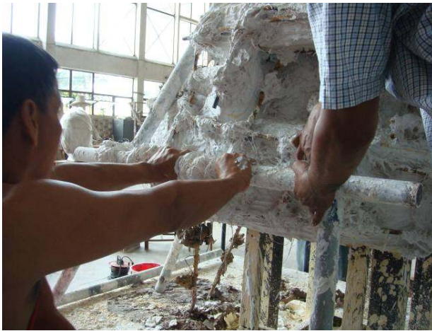
Figure 44 Attaching the zinc pipes for the strength and for stand.
