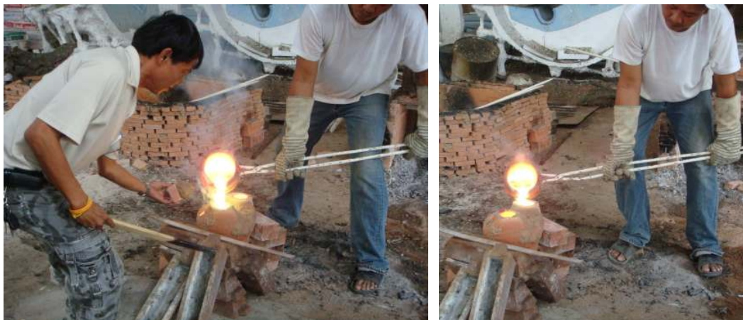
Figure 201 Pouring molten bronze on the air vent after the air is pushed out from inside bronze.
