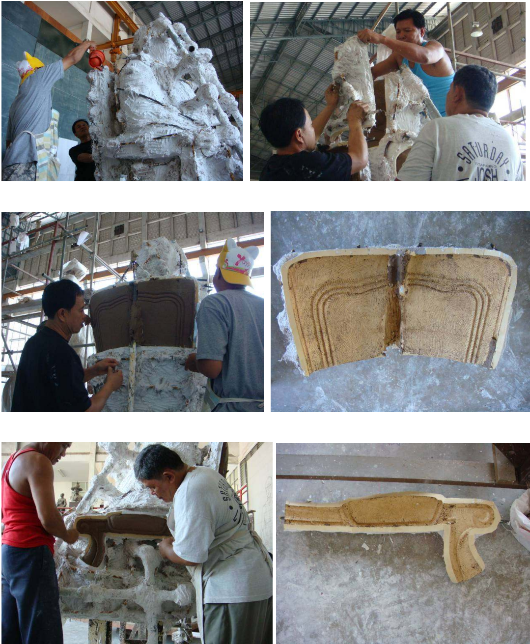
Figure 46 Separate plaster mould from the clay statue.
