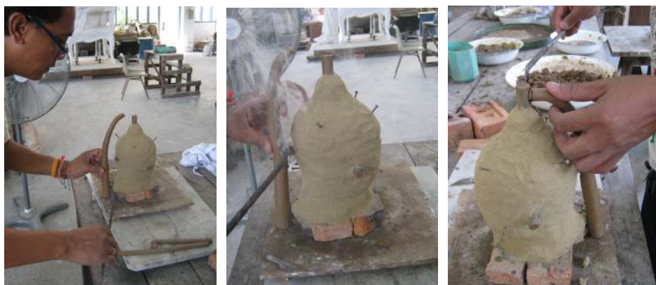
Figure 156 Attaching wax sprues.
