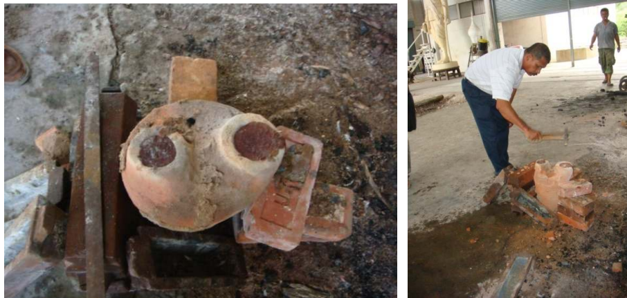
Figure 204 Breaking the mould after it cools.
