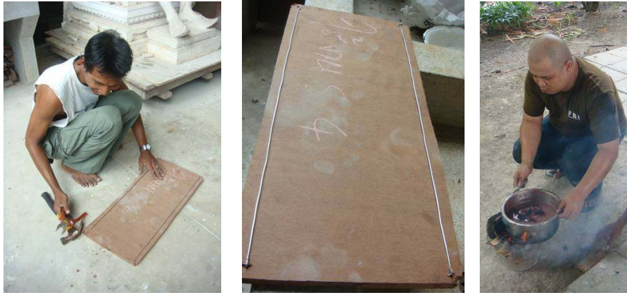
Figure 127 Prepare a board to roll to make wax sheet and melt wax on fire.
