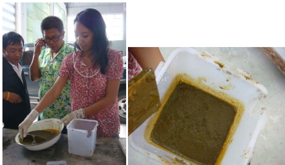
Figure 141 Mix soft clay dust with cow dung water.
