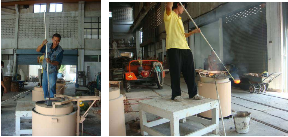
Figure 100 Stir and take out impurities.
