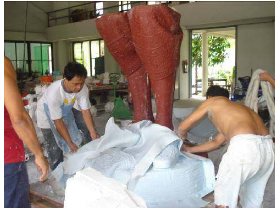
Figure 81 Peeling off the silicon sheet revealing the wax statue with the positive impression.
