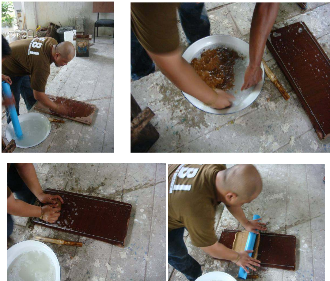
Figure 128 Melted wax poured in cold water and rolled on the board.
