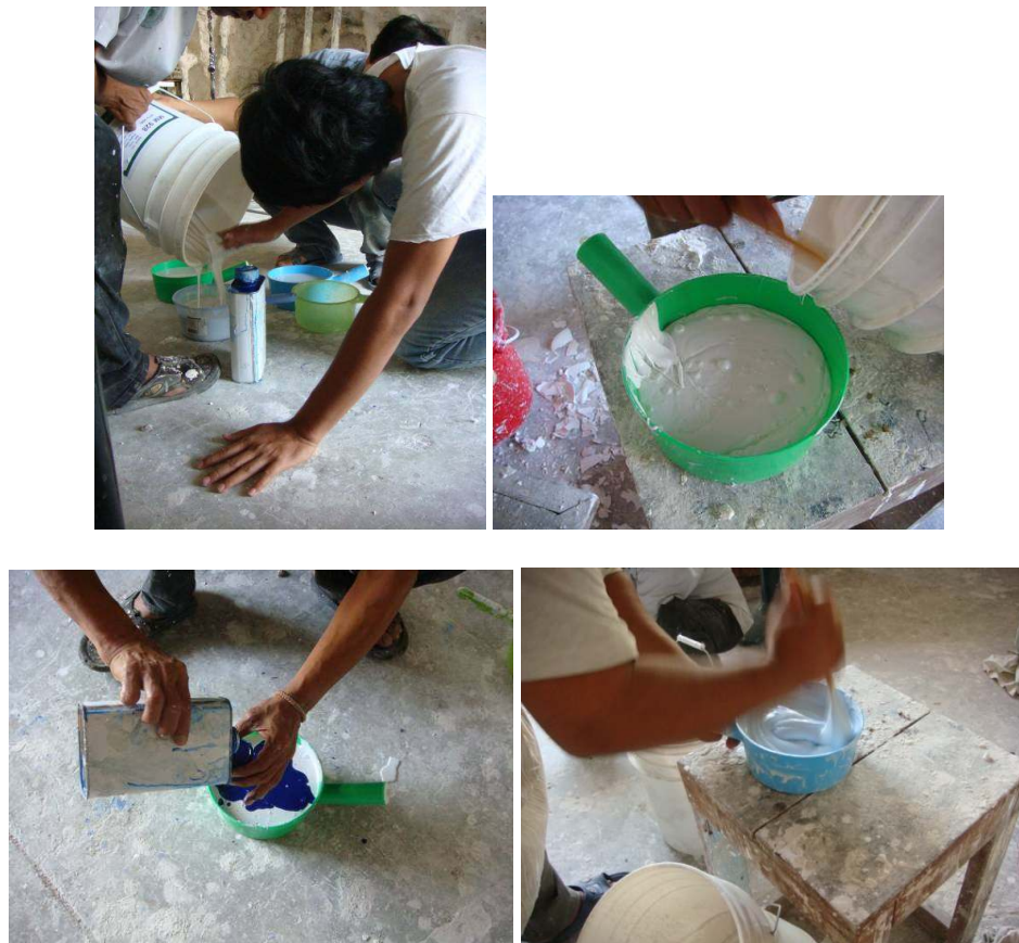
Figure 70 Mixing MM 928 Silicon Rubber and Standard Blue Catalyst.
