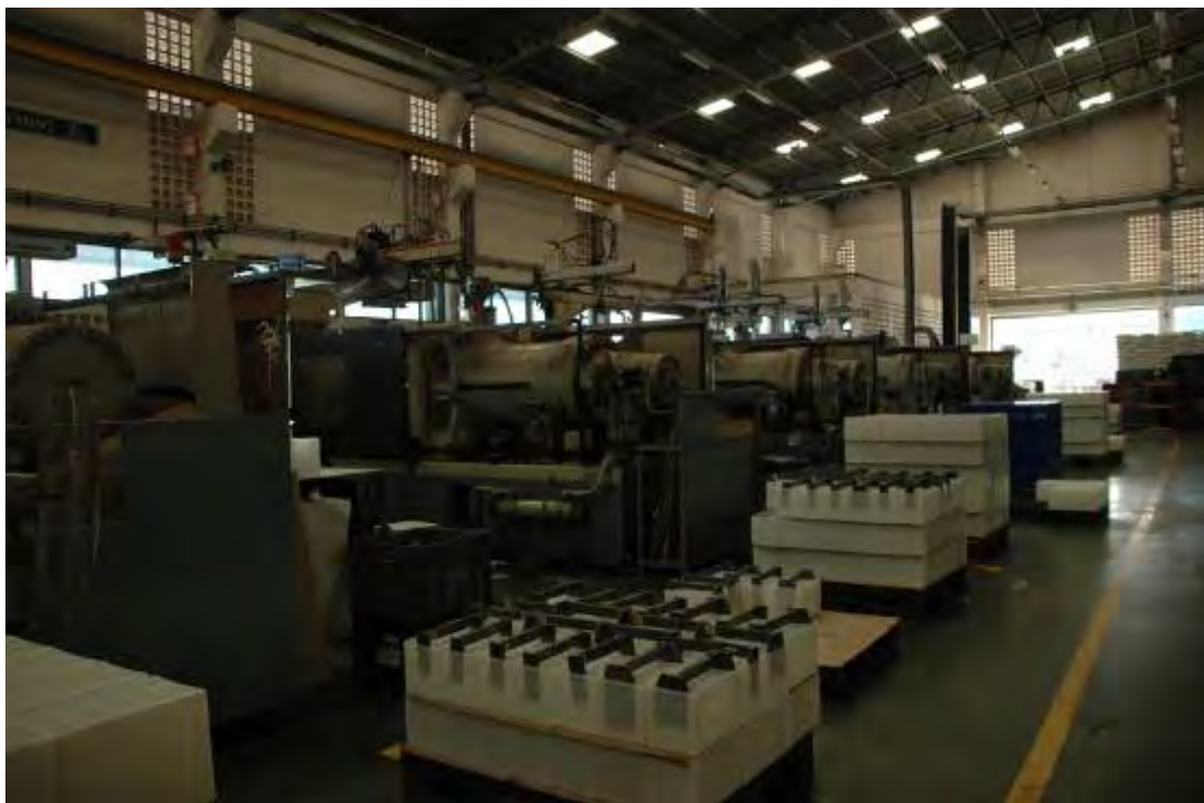
Figure 3.6: Plastic injection production line
