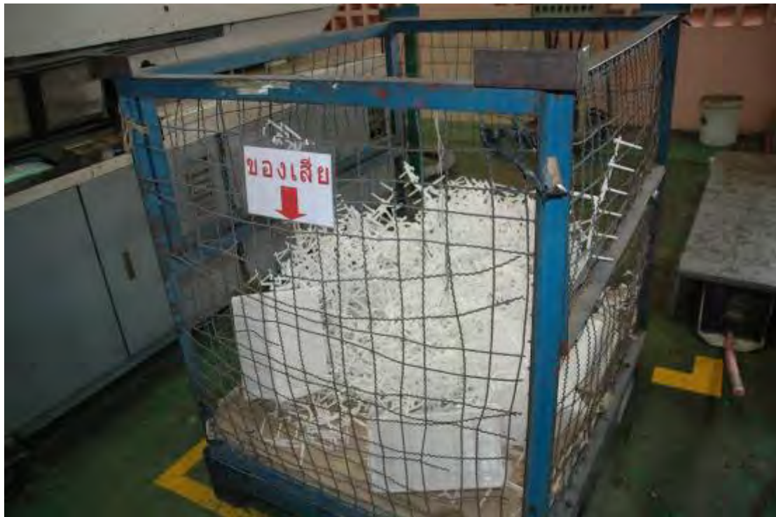
Figure 3.7 Plastic runners from production line
