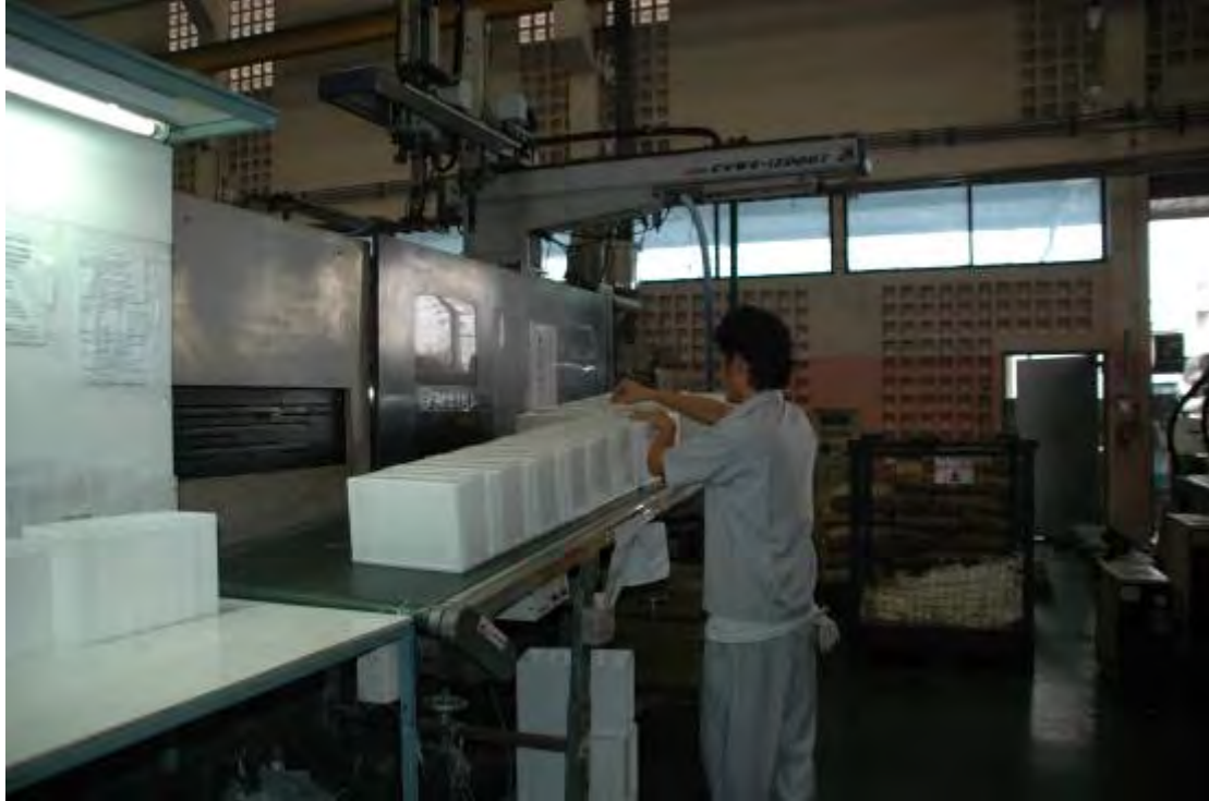
Figure 3.8 Operator check quality of injected part.
