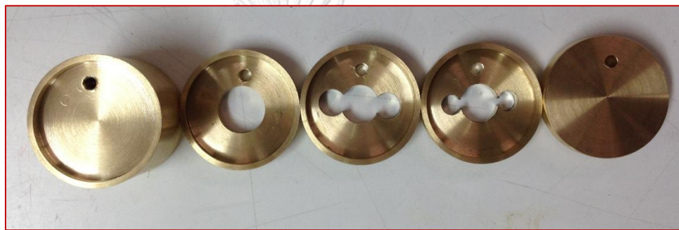
Figure 3.2 Copper collimator of aperture 2, 3 and 5 mm.
