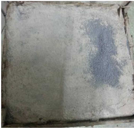
Figure 4. 17 After removal of lead powder from surface of dried shielding
