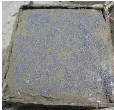
Figure 3. 16 Lead powder on surface of wet shielding
