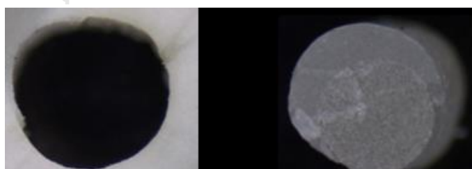
Figure162. Apical side of group9 sample1 shown adhesive failure between intra-radicular dentin and cement analyzed under Stereomicroscope at magnification of 45 (teeth after push out bond strength test (left), post after push out bond strength test (right))
