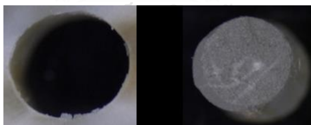
Figure144. Apical side of group8 sample2 shown adhesive failure between intraradicular dentin and cement analyzed under Stereomicroscope at magnification of 45 (teeth after push out bond strength test (left), post after push out bond strength test (right))
