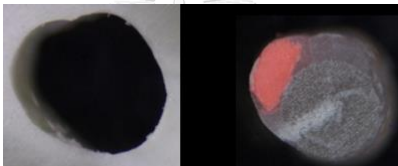
Figure 122. Apical side of group 7 sample 1 shown adhesive failure between intraradicular dentin and cement analyzed under Stereomicroscope at magnification of 45 (teeth after push out bond strength test (left), post after push out bond strength test (right))
