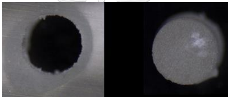
Figure110. Apical side of group6 sample5 shown adhesive failure between post and cement analyzed under Stereomicroscope at magnification of 45 (teeth after push out bond strength test (left), post after push out bond strength test ( right ))
