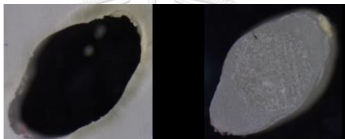
Figure131. Cervical side of group7 sample6 shown adhesive failure between intra-radicular dentin and cement analyzed under Stereomicroscope at magnification of 45 (teeth after push out bond strength test (left), post after push out bond strength test (right))
