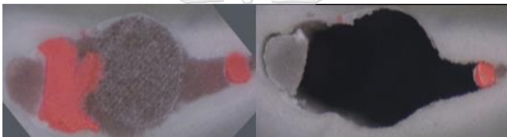
Figure65. Cervical side of group4 sample3 shown adhesive failure between intra-radicular dentin and cement analyzed under Stereomicroscope at magnification of 45 (before push out bond strength test (left), after push out bond strength test ( right ))
