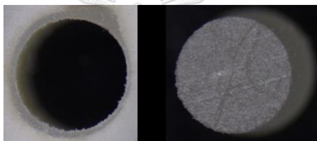
Figure113. Cervical side of group6 sample7 shown adhesive failure between post and cement analyzed under Stereomicroscope at magnification of 45 (teeth after push out bond strength test (left), post after push out bond strength test ( right ))
