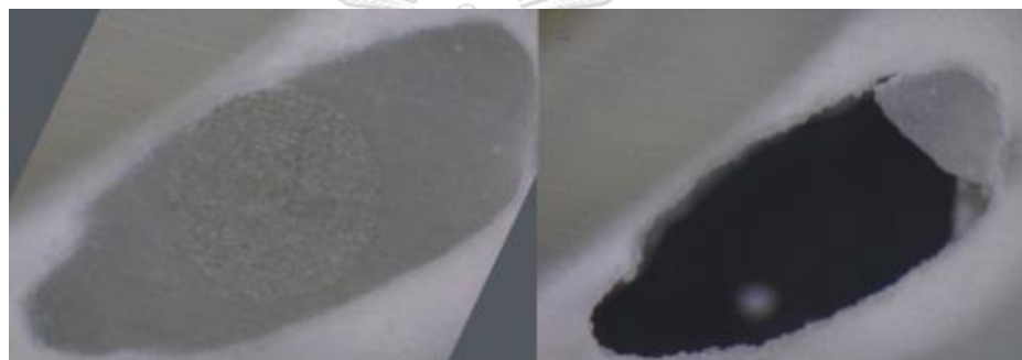
Figure71. Cervical side of group4 sample6 shown adhesive failure between intra-radicular dentin and cement analyzed under Stereomicroscope at magnification of 45 (before push out bond strength test (left), after push out bond strength test ( right ))
