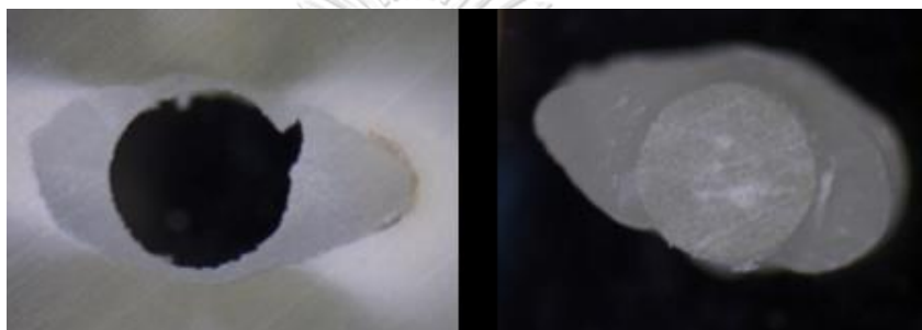
Figure83. Cervical side of group5 sample2 shown adhesive failure between post and cement analyzed under Stereomicroscope at magnification of 45 (teeth after push out bond strength test (left), post after push out bond strength test ( right ))
