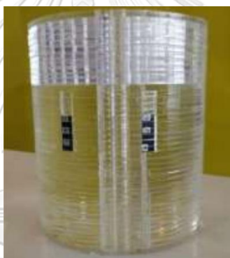
Figure I The nanoDot dosimeters were placed in the cylindrical phantom at the depth of 3 mm.
