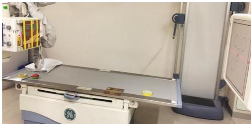
Figure 3 Set up detector for linearity and system transfer properties.
