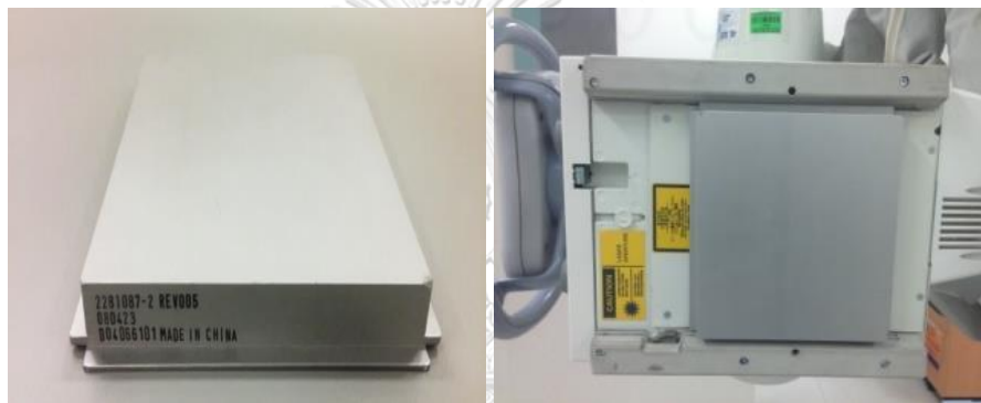
Figure 3.10 Insert flat field phantom into the collimator rail.
