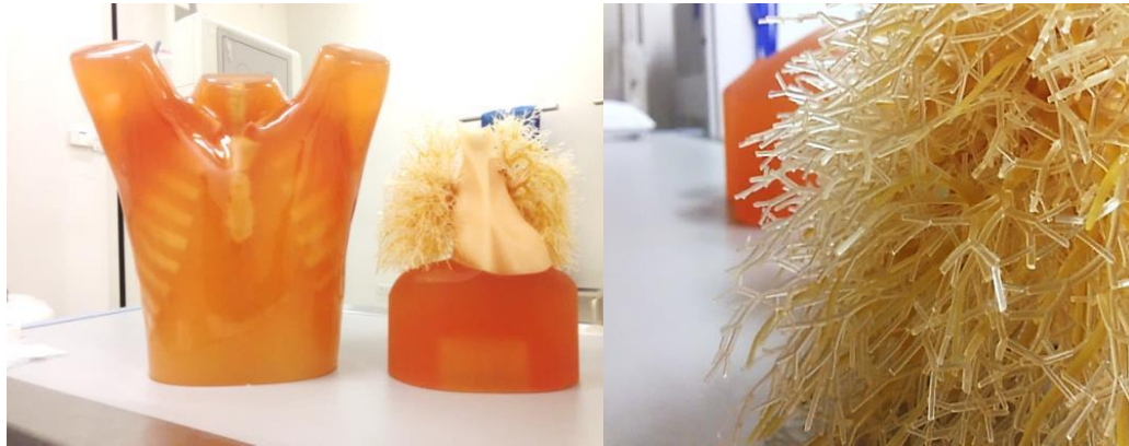
Figure 3.2 Multipurpose Chest phantoms N1 LUNGMAN.
