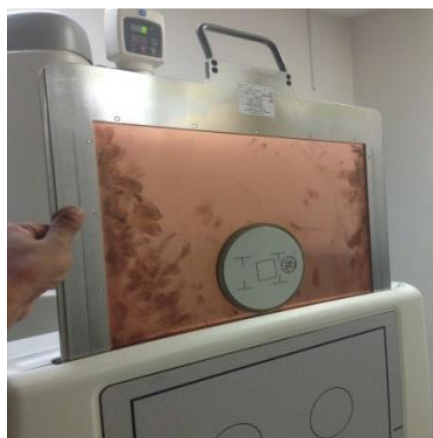
Figure 3.11 Insert the composite phantom into the grid holder.
