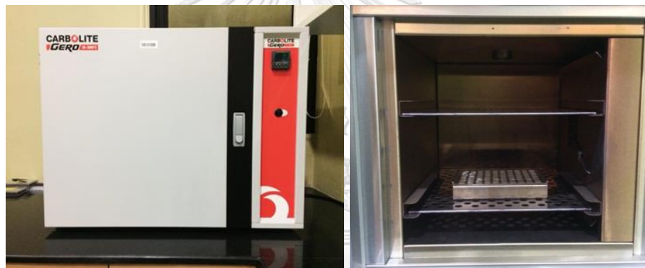
Figure 3.5 Laboratory oven used for annealing and pre heating of glass dosimeter.
