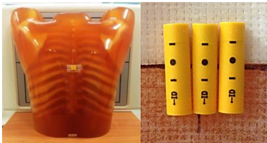
Figure 3.14 Setting of glass dosimeter for measuring ESD in phantom.
