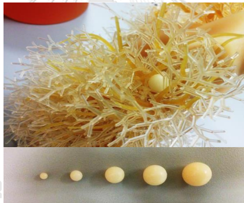
Figure 3.9 Five simulated nodules inserted in N1 LUNGMAN phantom.
