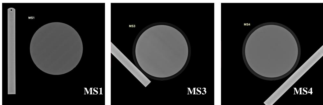
Figure 11 Place mesh and stainless steel ruler on the detector for any localized distortion, blurring and stitching artifacts.
