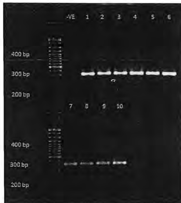
Figure 4.1 A photograph of an agarose gel electrophoresis showed some amplified products from malaria parasite samples. The gel electrophoresis condition was 1.5% (W/V) agarose in 1XTBE buffer processing under 80 voltages for 30 mins. After staining with ethidium bromide, the products were detected by UV transilluminator (UVP Bioimaging systems, AutoChem system). The amplified product size was compared with 100 bp DNA standard ladder marker (BioExcellence, Thailand).
