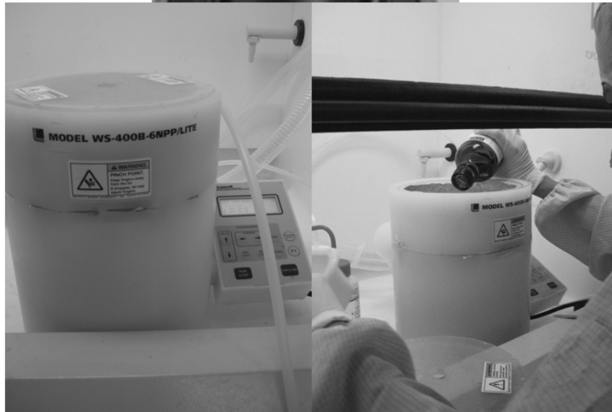
Figure 8. Photograph of the mould fabrication process according to the standard MEMS techniques illustrating (A) piranha etching ( \text{H}_2\text{SO}_4 & \text{H}_2\text{O}_2 ) and (B) a photoresist material (SU-8 2100) spun on the silicon wafer.
