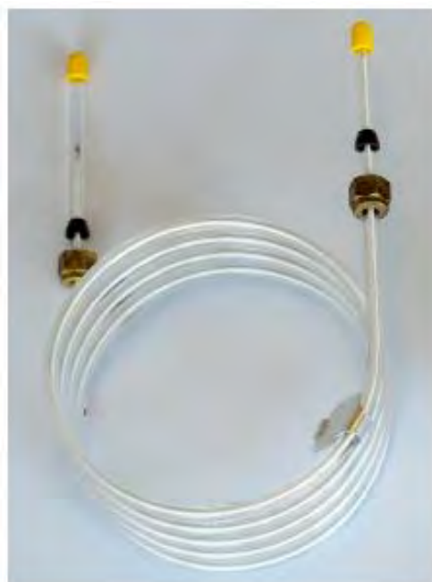
Figure 2.16 Packed column of gas chromatography (Piantanida et al. , 2014).
