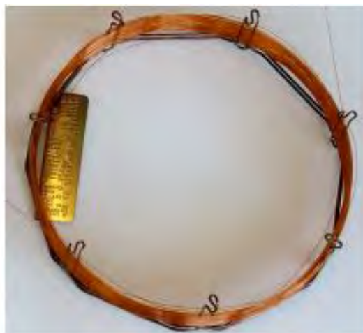
Figure 2.15 Capillary column of gas chromatography (Piantanida et al. , 2014).
