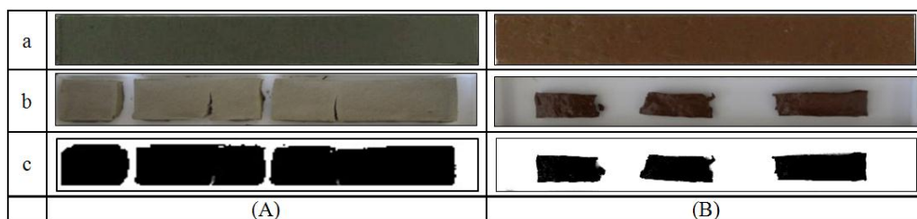
Figure 3-4: Typical photograph of soil specimen surface area seven days before and after air dry (a = before air-dried, b = after air-dried, c = binarised to black and white after image thresholding on air-dried specimens).
