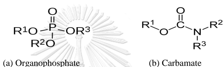
Figure 2. 7 The general structure of organophosphate and carbamate pesticide form
