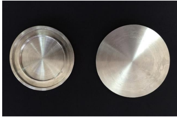
Figure 3. Circular mold recommended by ISO 20795-1 (2013)
