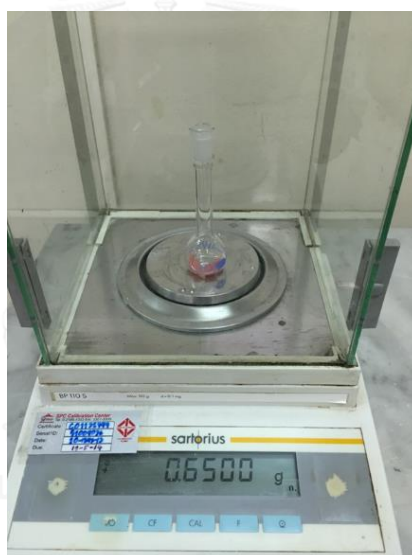
Figure 9. Each sample was weighed by the Sartorius BP1105 digital scale
