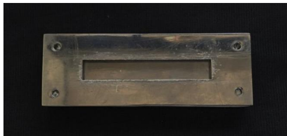
Figure 5 Mould for flexural strength and modulus tests: stainless steel mould with 64 mm in length, 10 mm in width, 3.3 mm in height, ISO 20795-1
