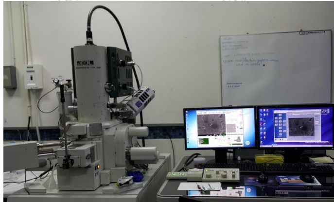
Figure 7: Scanning Electron Microscope (SEM; JSM-6610LV, JEOL, Tokyo, Japan) and Energy Dispersive X-Ray Spectroscopy (X-Max N 50, Oxford instruments, Oxfordshire, United Kingdom)
