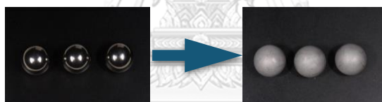
Figure 6 Step 4 : Drilled model with cylinder stone bur in 3mm depth to be the area of calibrated metal sphere balls.
