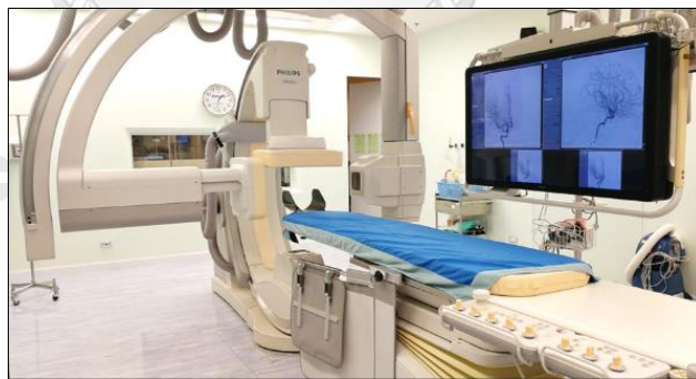
Figure 3.6 Digital R/F biplane system (Philips Allura Clarity Xper FD20/15)
