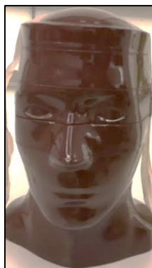
Figure 3.10 Anthropomorphic CT head phantom
