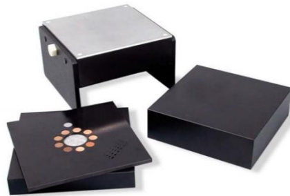
Figure 3.5 The CIRS 903 R/F QA phantom (CIRS Inc., Virginia, USA)
