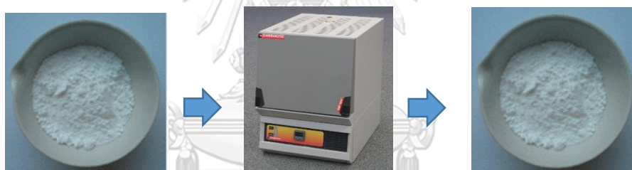
Heat treatment in air at 600-900°C for 5h
