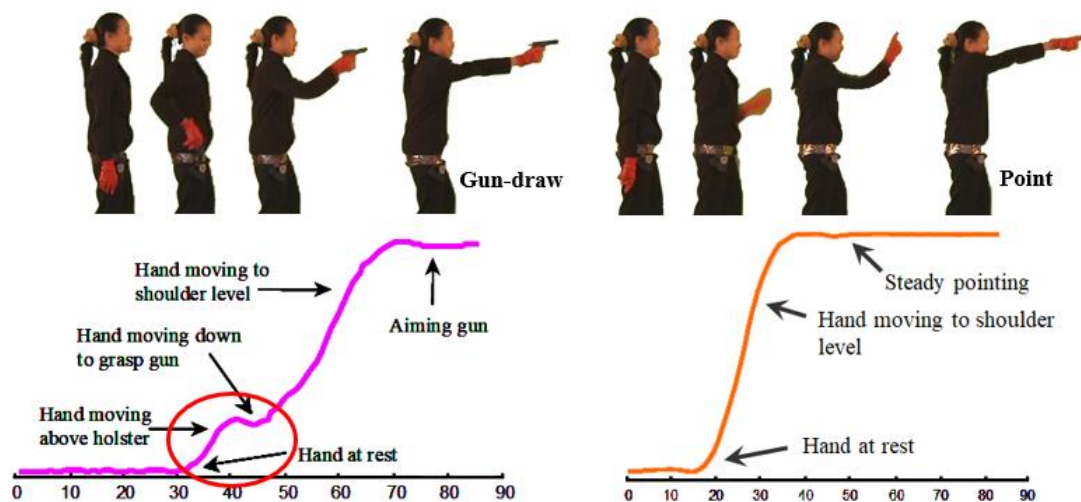
Figure 2 A comparison between time series sequences that created from motion of the actions in the video of a person holding and the pointing a gun (Gun time series) and a person pointing a finger (No gun time series).
