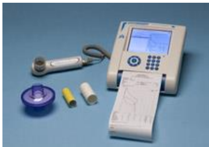
Figure 3.4 FUTUREMED Discovery-2 Diagnostic Spirometer
