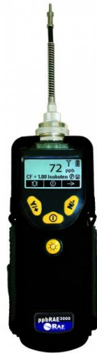
Figure 3.3 ppbRAE3000 VOC monitor
