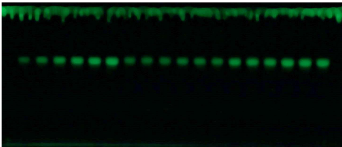
Figure 36 The TLC image subtract background from UV 254 nm picture using imageJ software; mangiferin standard (tract 1 – 6) and A. crassna leaf extracts from 15 different locations (tract 7 – 21)
