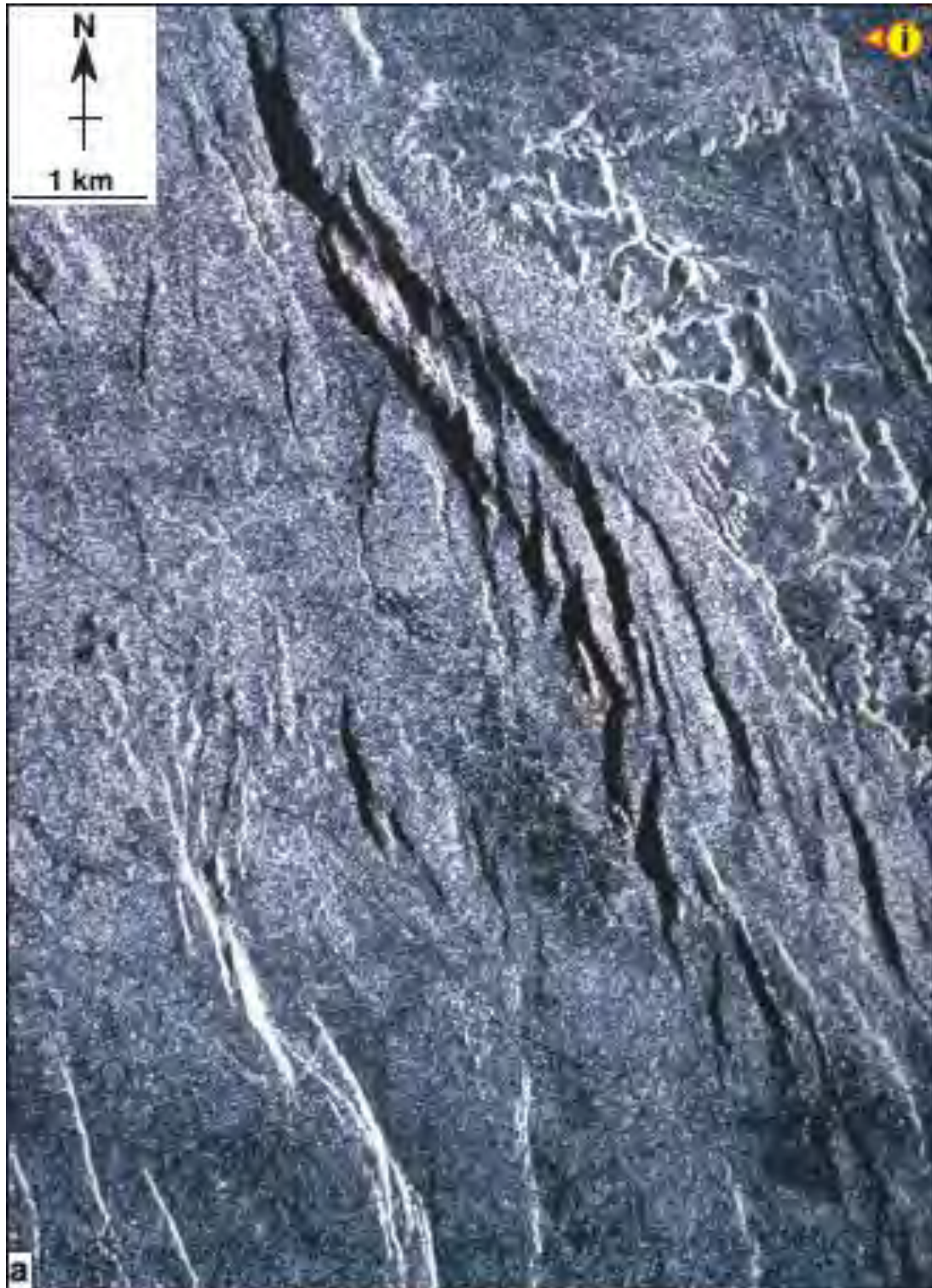
Figure 5.2a Radar image of the volcanic tablelands, Bishop, California. The image shows a series of en echelon marginal faults in the Bishop running obliquely across the image with north-south-oriented interior faults in the center left of the image (modified after McClay et al., 2002). Continued.
