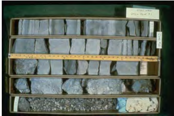
Figure 1.2 Core samples contain missing intervals because the rocks are broken into fragments (USGS, 1999)
