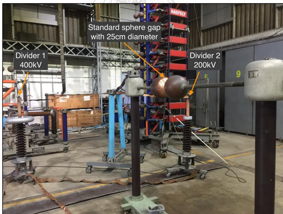
Figure 1-1 The standard sphere-gap with 25cm diameter is used for the performance check of voltage dividers ratio.
