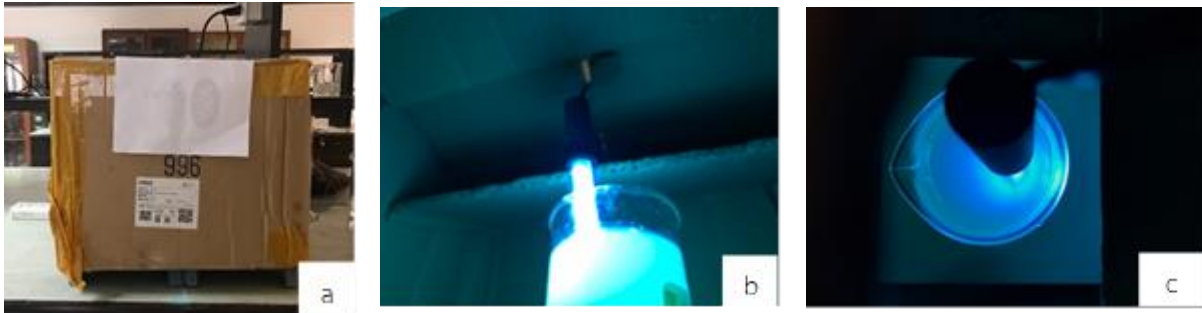
Figure 3.7 Electronic effluent treated by photocatalytic using \text{TiO}_2 in (a) front, (b) below and (c) top
