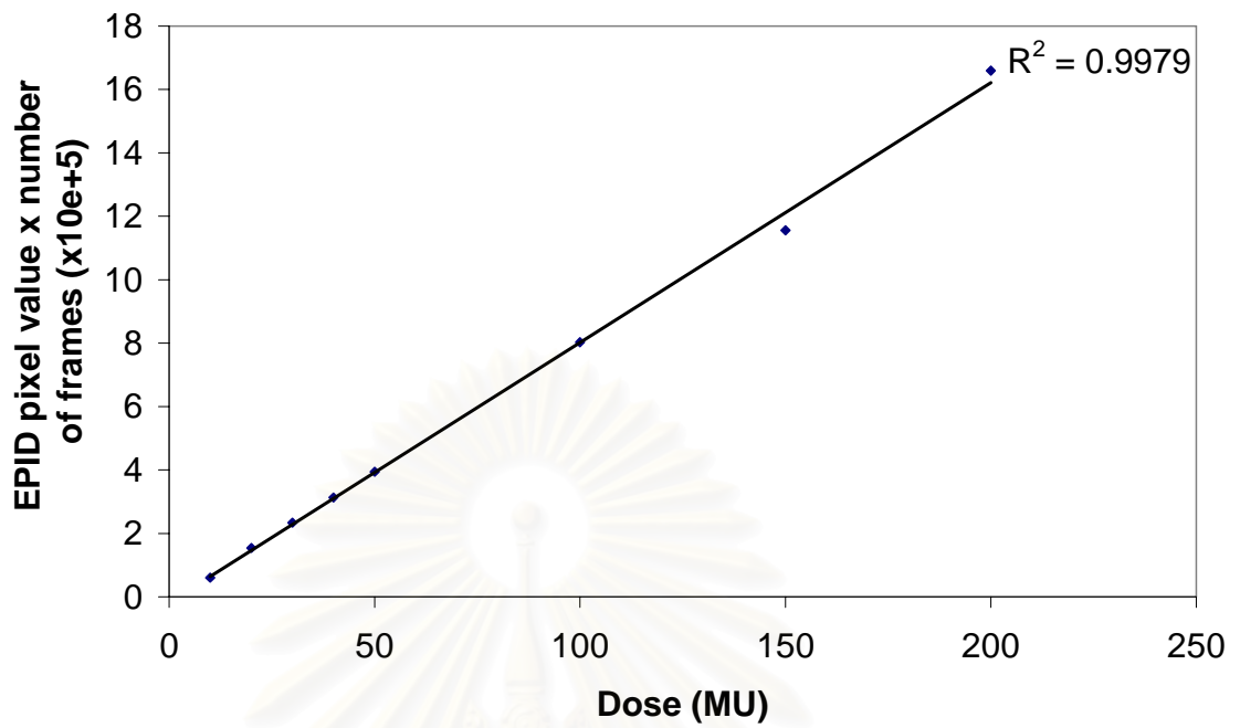
Figure 6.4 The linearity of EPID with integral dose in 10 x 10 cm 2 field size.
