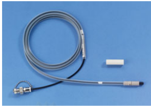
Figure 5.5 0.125 cc ion-chamber (Well-hofer Dosimetrie, Schwarzenbruck, Germany)
