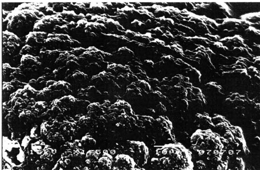
Figure H-3 Scanning electron micrograph of the coating admicelled rubber (with 100 mM PPy) by using electrochemical method magnification 1,500/15 kV.
