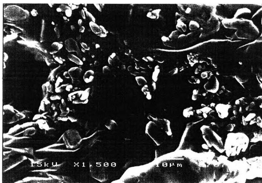
Figure H-14 Scanning electron micrograph of the coating admicelled rubber (with 800 mM PTh) by using electrochemical method magnification 1,500/15 kV.
