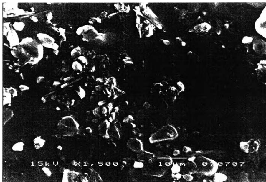
Figure H-13 Scanning electron micrograph of the coating admicelled rubber (with 500 mM PTh) by using electrochemical method magnification 1,500/15 kV.
