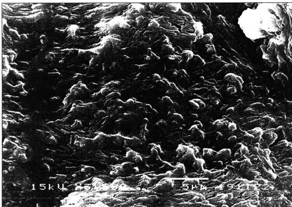
Figure 7.13 Scanning electron micrograph of the coating admicelléd rubber (EB2) by using electrochemical method magnification 3,500/15 kV.
