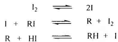
Figure 7.40 Reactions leading to the formation of conjugated sequences in polybutadienes following treatment with Iodine.
