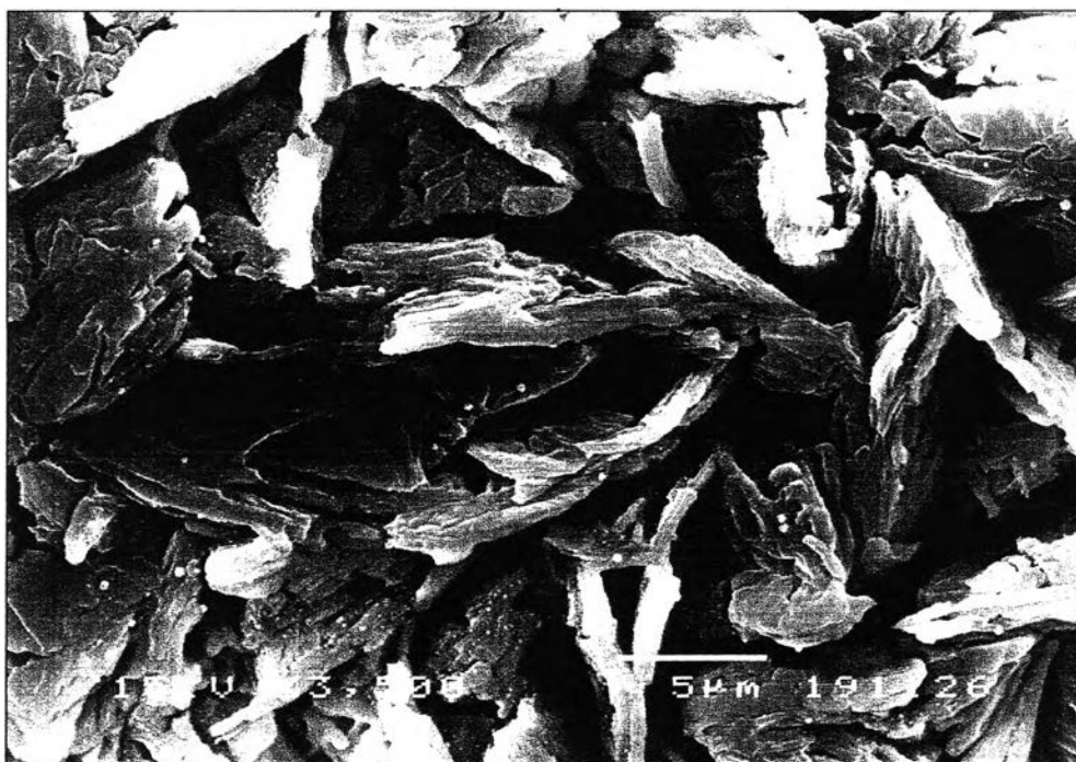
Figure 7.14 Scanning electron micrograph of the coating admicelléd rubber (EB80) by using electrochemical method magnification 3,500/15 kV.
